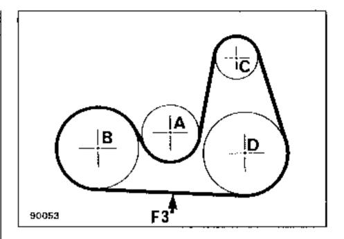
Coolant pump-Power steering- alternator belt
