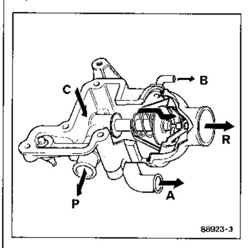
The thermostat (figure 2) is "open". It allows the coolant from the cylinder head (circuit C) to pass to the radiator (circuit R) and closes off circuit P, which formerly connected the cylinder head (circuit C) to the coolant pump.
