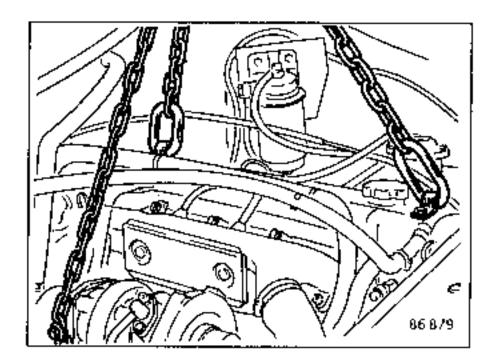
Lift out the engine-gearbox assembly REFITTING (special points)
