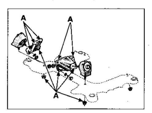
Remove the engine using tool Mot.878.
