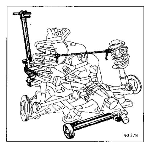
Secure the spring-shock absorber assemblies with string.
