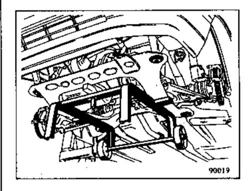
Lower the lift until the dummy frame makes contact with the floor.
