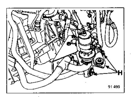
Fit the 2 clamps Mot.453-01 to the power steering reservoir output hoses.
