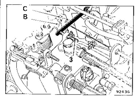
Check the initial idling speeds, with and without the lum feeler gauge, and if the speeds have altered, repeat the adjustments (b, c and d).
