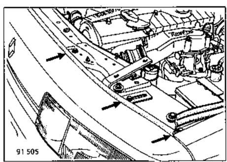
the upper cross member including the intercooler, clips (A) and bolts (B),
