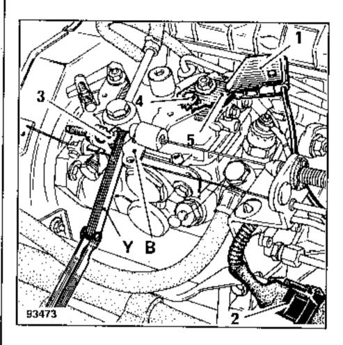
Use an ohmmeter or a test lamp connected to pins B and C on connector (2).
