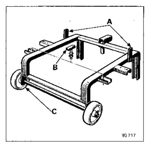
Secure the dummy sub-frame 1040-01 under the engine sub-frame.
