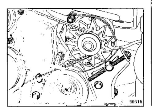
Remove the cable protector from the timing gear casing and pull it forwards.
