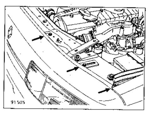
the upper cross member together with the intercooler, clips (A) and bolt (B),
