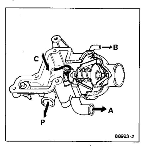
The thermostat (Figure 1) is closed and the coolant from the cylinder head (circuit C) is passed back to the coolant pump through circuit P, the heater through circuit A and the cold starting system (Bosch pump) followed by the "hot" expansion bottle through círcuit (B).
