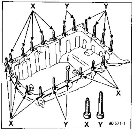
The screws are of the Torx type and tool Mot. 1 063 must be used.
