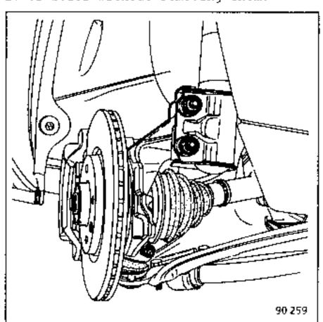
Tilt the stub axle carriers and extract the drive shafts from the sun wheels.
