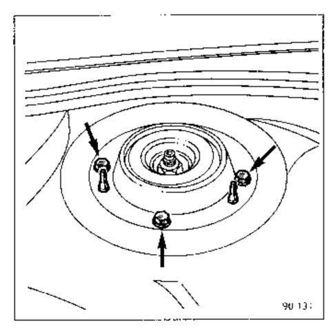
Remove the nut from the suspended flexible mounting and free the screwed rod from the flexible bush by knocking it with a bronze drift.
