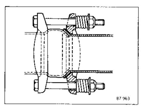
The spherical joint is sufficiently tight as soon as an effective seal between the 2 pipes is obtained.
