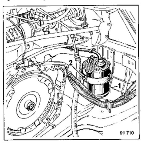
The canister bleed solenoid valve is mounted, together with the pressure sensor, on the injection computer protective casing.
