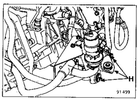
Place clamps Mot.453-01 on the power steering reservoir output hoses.
