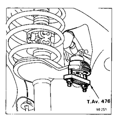
the nuts from the steering ball joints and extract the ball joints using tool T.Av.476.
