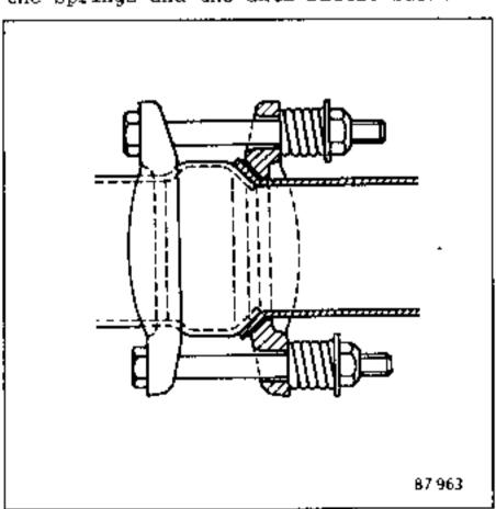
The joint is sufficiently tight as soon as an effective seal is obtained between the two pipes.
