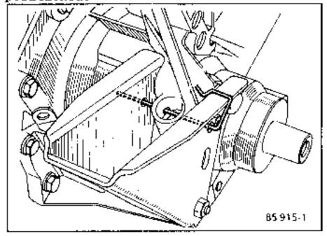
Adjust the accelerator and choke cables.
