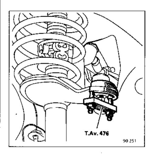
Remove the upper bolts securing the lower ends of the shock absorbers and loosen the lower bolts without removing them.
