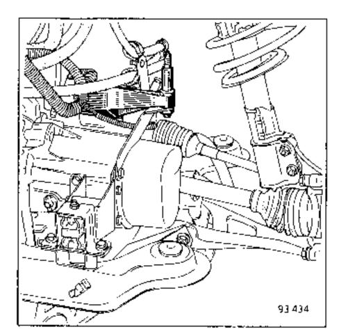
Lift the vehicle body and take out the power unit assembly. Secure the spring-shock absorber assemblies with string.
