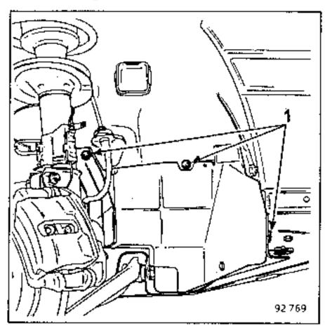
The tie bars securing the sub-frame to the body.
