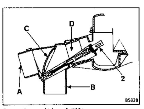
Remotely positioned Filter
