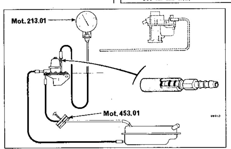
A degassing valve is fitted between the fuel pump and the carburettor to improve starting when hot.
