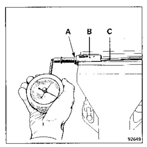
Grip tool Ele. 346 in a vice after first removing its plug. Apply the cylindrical part of tool B.Vi.906 to the end of the sliding part. The shoulder (A) should be flush with the plunger body (B) when the pointer shows 3 dan. If it is not, adjust screw (C) to increase or reduce the spring pressure.
