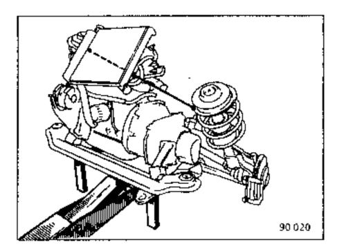
Secure the spring-shock absorber assemblies with string.
