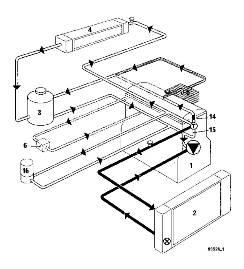
Flow through oil cooler, coolant pump (AC)
