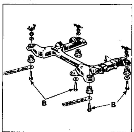
Take out the power unit assembly by lifting the body.
