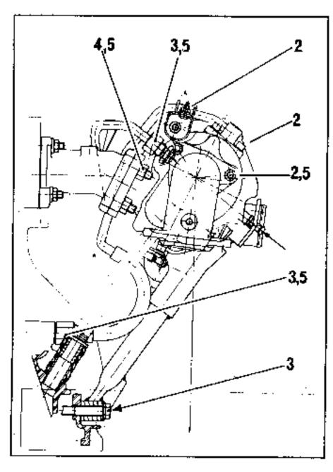
Fill the turbocharger with engine oil through the input hole.
