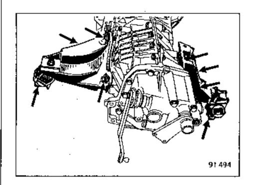
Secure the computer unit and the power steering reservoir to the engine.
