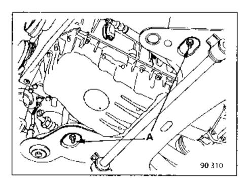
Lift the engine, either by means of an engine lifting cross piece FACOM WM103, or with a workshop crane secured to the front lifting lug.
