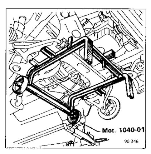
Lower the vehicle, fitted with sub-frame Mot. 1040-01 to the ground.
