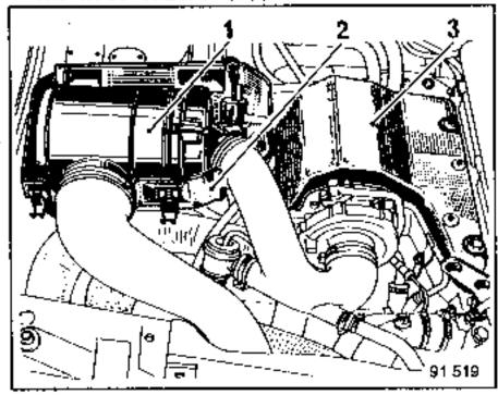
the turbocharger air input and output ducts.
