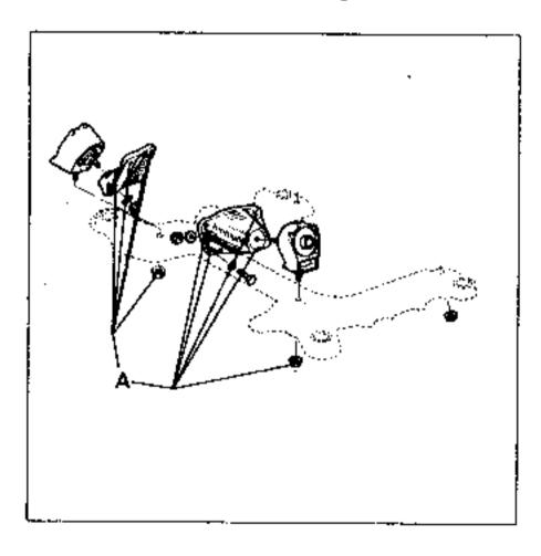
Remove the engine using tool Mot.878.
