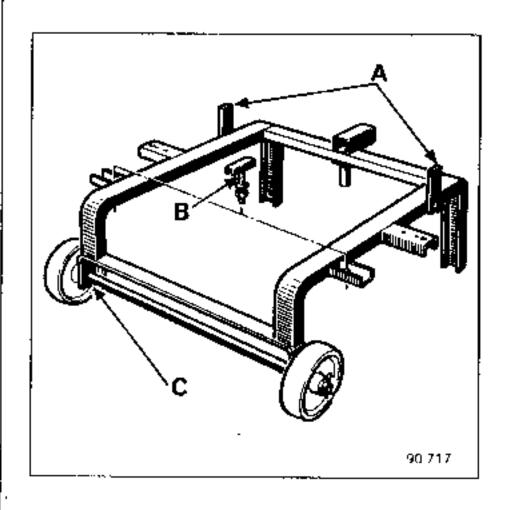
Secure frame Mot. 1 040-01 under the sub-frame.
