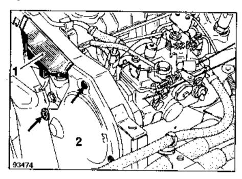
Remove the plastic cover (1) and the pressed steel casing (2).
