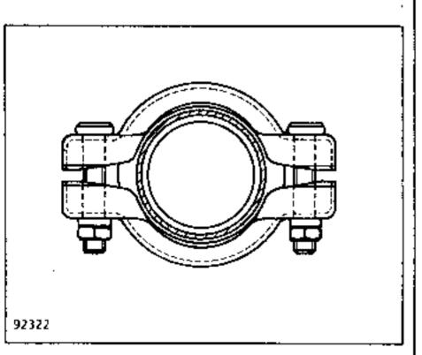
Tighten the clamp bolts to the specified torque: 8mm Ø bolts:
