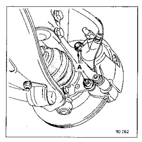
the steering ball joints using tool
