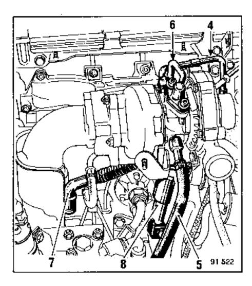
Pinch flat the coolant hoses (4) and (5) and disconnect them (clamps Mot. 453-01).
