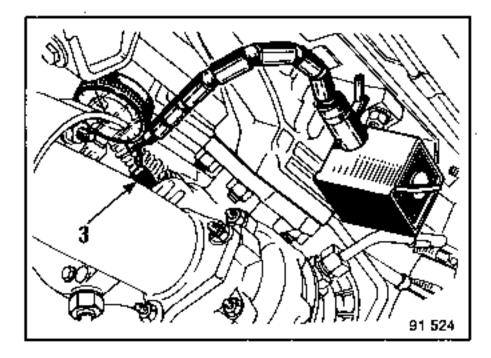
Slowly increase the pressure until the adjusting rod has moved by 0.38 - 0.02mm and note the pressure gauge reading which should be within the checking values stated.
