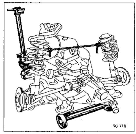
Secure the spring-shock absorber assemblies with string.
