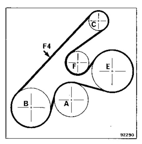
Coolant pump-compressor-alternator belt
