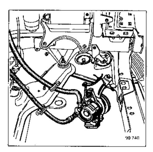
Pit the engine, ensuring that the clutch fork lugs are correctly positioned behind the shoulder on the withdrawal bearing (the bearing is an integral part of the clutch unit).
