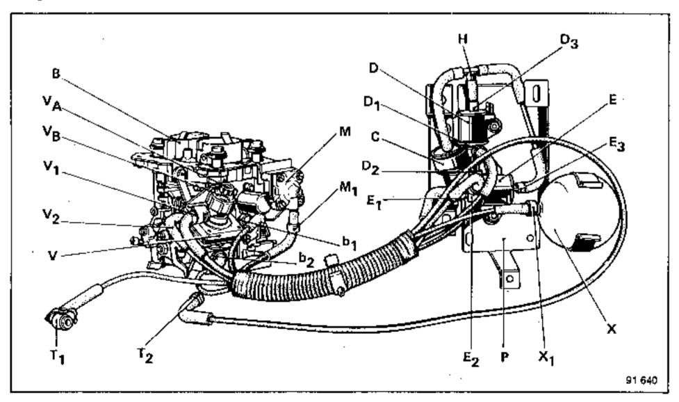
Pneumatic control system circuit diagram:
