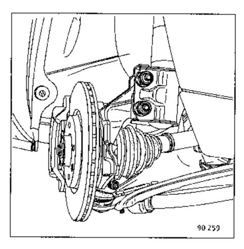
Tilt the stub axle carriers and free the drive shafts. Remove the bolts from the gearbox mount: ing pads.
