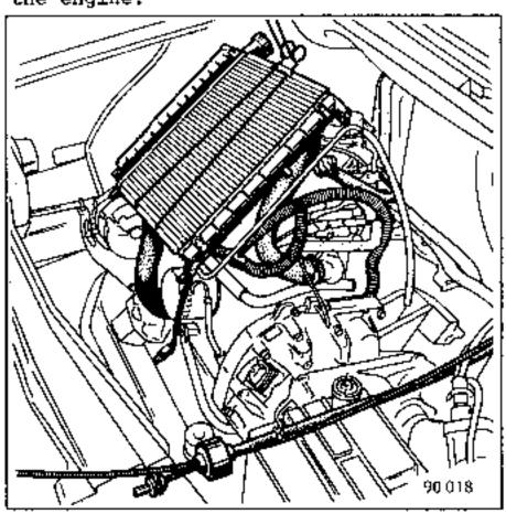
Fit the 2 clamps Mot. 453-01 to the heater hoses, then disconnect them from its inlet and outlet sides.
