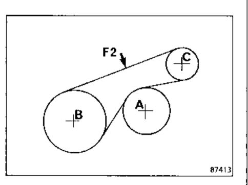
Coolant pump-alternator belt
