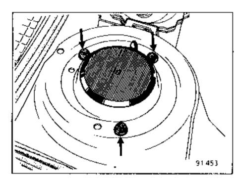
Remove the sub-frame securing bolts.
