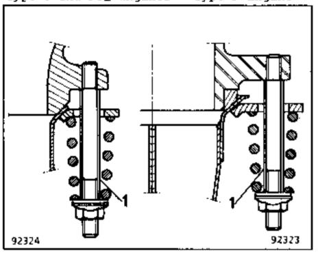
NOTE: the exhaust down pipes are fitted with spacers (1) which determine the spring pressure. Tighten until making contact with the spacers.
