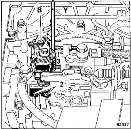
The system is adjusted by moving the micro switch (1) on its support.
