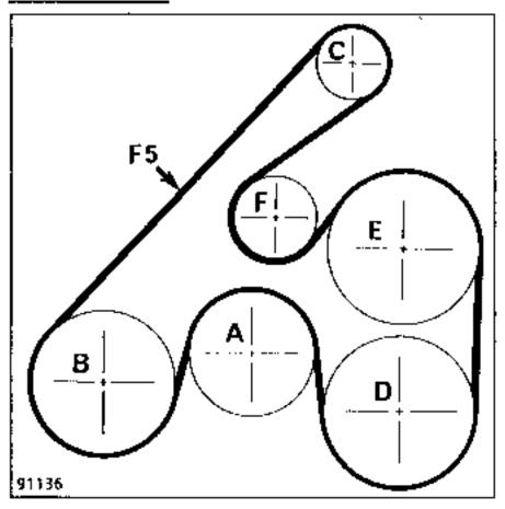
Coolant pump-power steering Compressor-alternator belt
