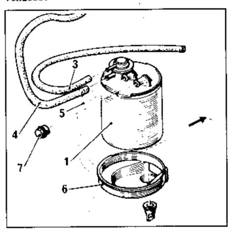
1 - Fuel vapour absorption canister
