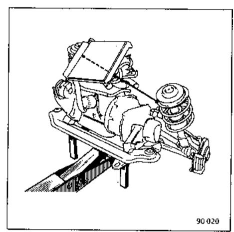
Secure the spring-shock absorbers in place with the string.
