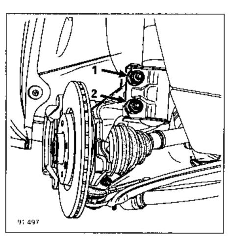
Tilt the stub axle carriers and disconnect the drive shafts.
