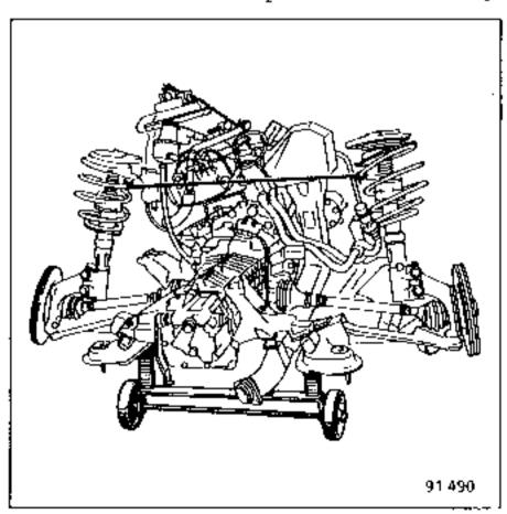
Secure the spring-shock absorber assemblies with string, and also the injection unit.
