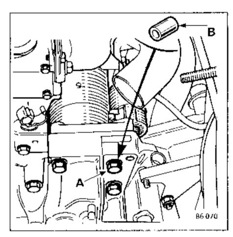
the method of tightening the exhaust pipe clamp. Tighten the nuts until the springs are coil bound and then loosen them by one and a half turns.
