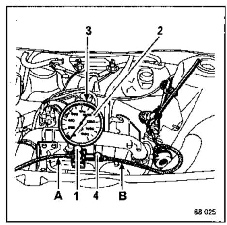
Before using the equipment, zero the pressure gauge (screw 3), fully unscrew the pressure reducing valve screw (1) and the leak screw (4) and connect the inlet pipe (A) to the compressed air supply.
