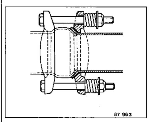
ESSENTIAL: Replace the thermoplastic seal each time the joint is disconnected by an anti-rattle ring, reference 60 25 071 196. The joint is tight enough as soon as the seal between the two pipes is complete.
