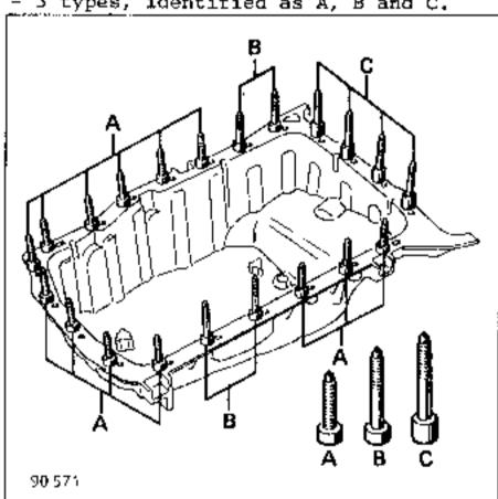
Do not refit the engine to the vehicle before tightening the sump screws.
