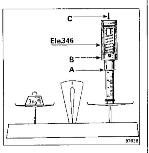
Apply a force of 3 dan (weight of 3 kg) to the tool. The shoulder (A) should be flush with the plunger body (B). If it is not, turn the screw (C) to increase or reduce the spring pressure.
