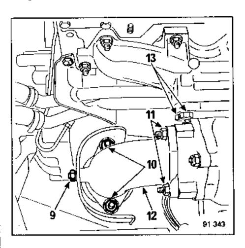
Using combination spanner FACOM No. 40, modified as shown in the illustration below, unscrew the turbocharger securing nuts (13) and remove it.
