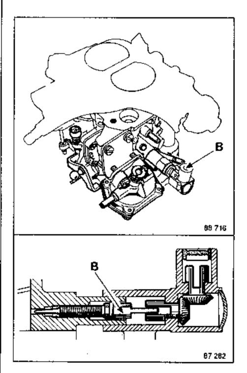
Method of Adjusting the Idling Speed: SOLEX 28 x 34 Z 10
