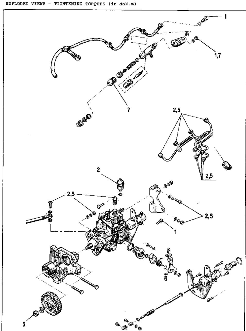
EXPLODED VIEWS - TIGHTENING TORQUES (in dan.m)
