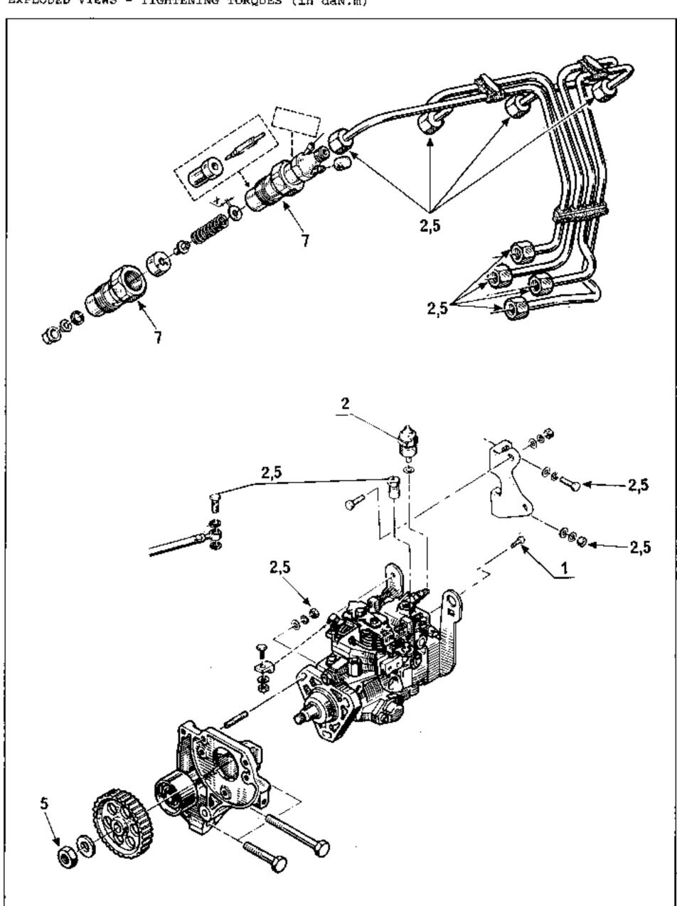
EXPLODED VIEWS - TIGHTENING TORQUES (in dan.m)
