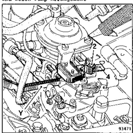
The adjustment is carried out by moving the cam on the throttle lever.
