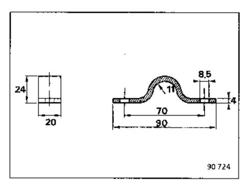
Use tool  ${\tt Mot.878}$  securing the engine-gearbox assembly at the lifting lugs.
