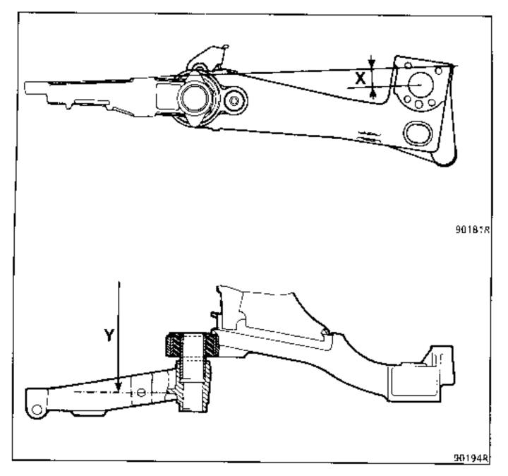
In this position, fit the bearing using components (A) and (C) from tool T.Ar. 1056 until dimension Y = 1285  $\pm$  1 mm  $\,$  is obtained between the bearing centre lines
