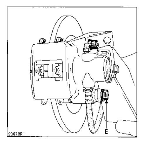
Unscrew the calliper on the hose (place a container underneath to catch the fluid).
