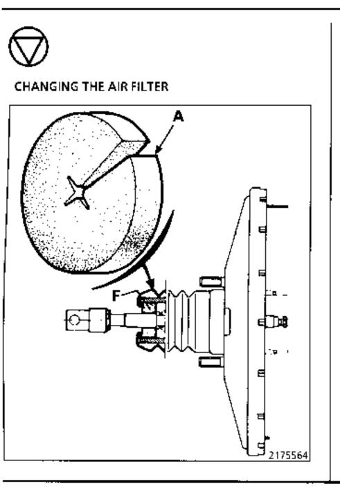
It is not necessary to remove the servo unit in order to change the air filter (F).
