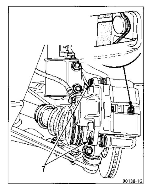
The pad to which the wear warning light wire is connected is fitted on the inside.
