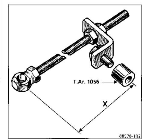
Fit the two tools in place of the shock absorbers.
