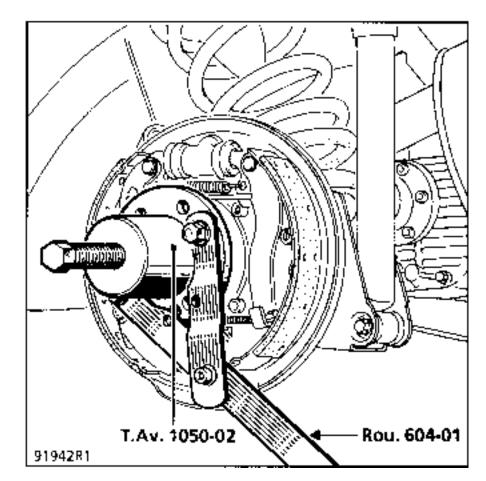
Using tools T.Av. 1050-02 + M.S. 580 take out the hub and recover the bearing inner track ring.
