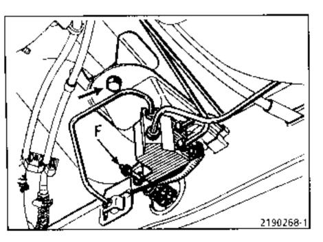
Uncouple the compensator from its support.
