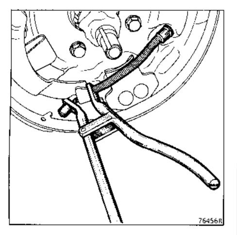
Using a tool such as the end of a valve adjusting spanner, remove lateral shoe spring (R), holding connecting rod (T) against brake back plate (E).
