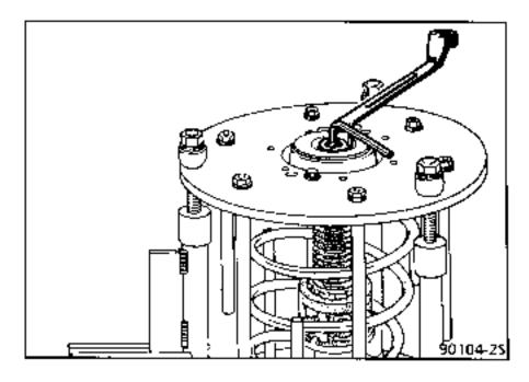
Torque tighten the nut.
