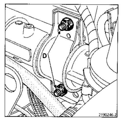
the PVC collar holding the bulkhead gaiter on the steering box. Free the steering box, moving it towards the front and remove :
