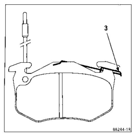
**NOTE :** these vehicles are equipped with pads with offset linings. .
