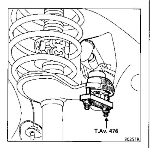
the two bolts (1) securing the bottom of the shock absorber,
