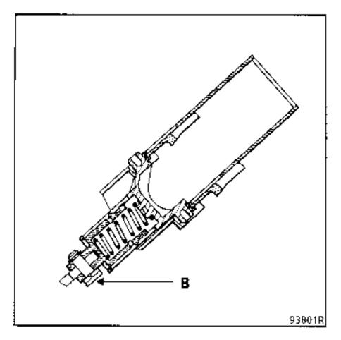
Remove tool Emb. 1082 and refit the circlips on the shaft.
