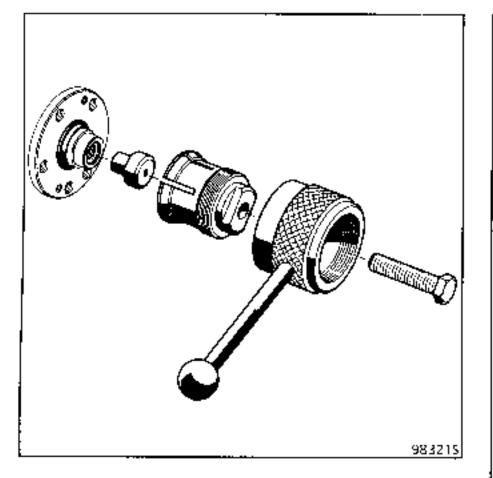
Disconnect the steering arm using tool T.Av. 476.
