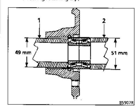
the bearing, using a piece of tubing (1).
