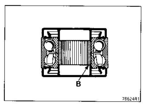
Do not rest on the inner track ring, otherwise the bearing might be damaged since great force is required to fit the bearing.
