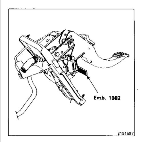
Remove the circlip and rollpin from shafts (8) and (C).
