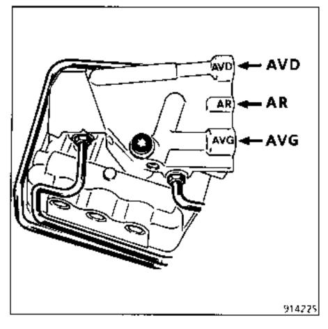
V - HYDRAULIC UNIT CONNECTOR PINS
