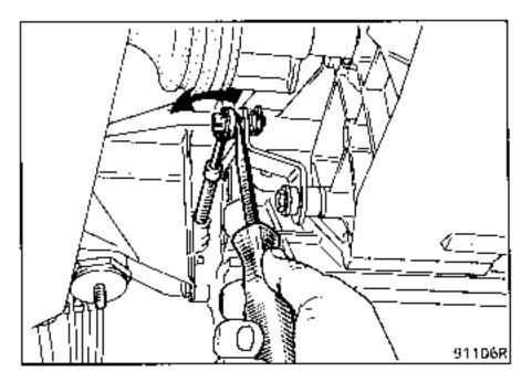
Lower the engine/gearbox cradle by **15 mm by** unscrewing the two rear mountings.
