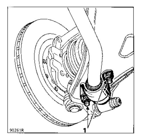
Compress the front of the vehicle and secure the two bearings (2) on the cradle.
