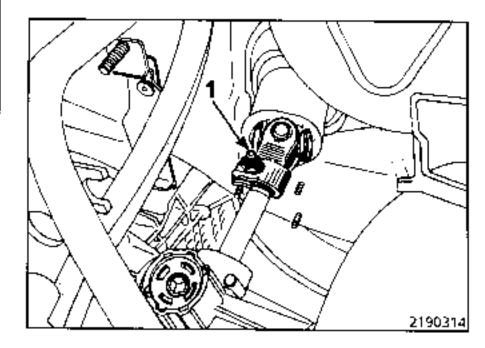
Tilt the steering box downwards and remove it from the righthand side.
