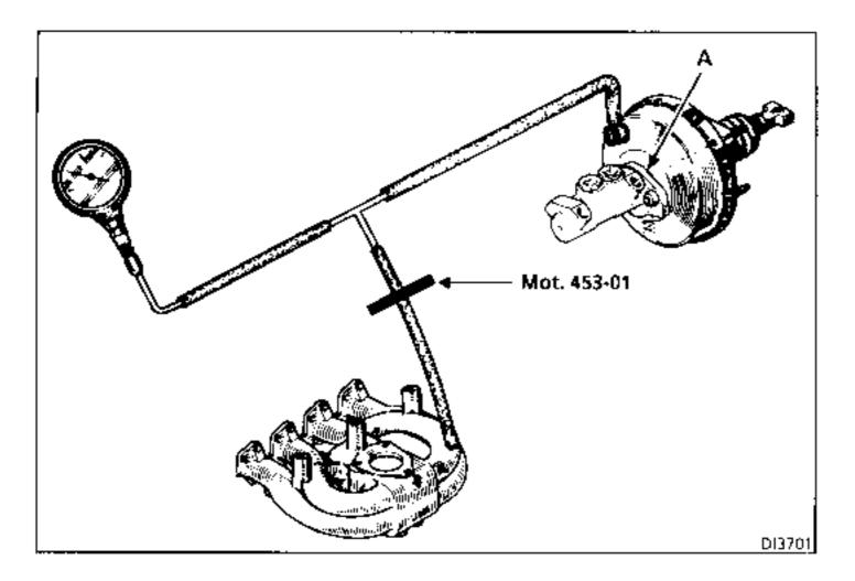
The test for loss of vacuum in the brake servo must be carried out with the unit on the vehicle and with the brake hydraulic circuit operating correctly.
