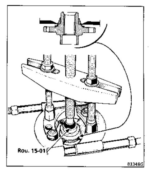
Remove the circlips holding the bearing on the arm.
