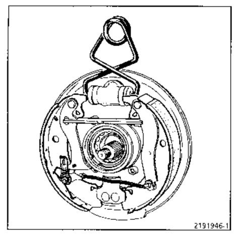
Remove the grips on the wheel cylinder pistons and then refit the side retaining springs (2) using tool Fre. 826.
