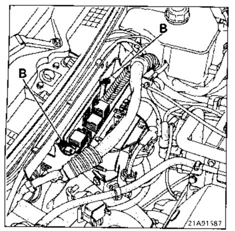
Move the wiring loom away and take out the relay plate.
