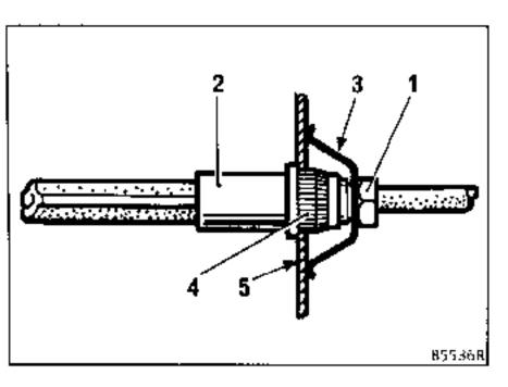
Unscrew the hose from the calliper. Release the calliper if necessary.
