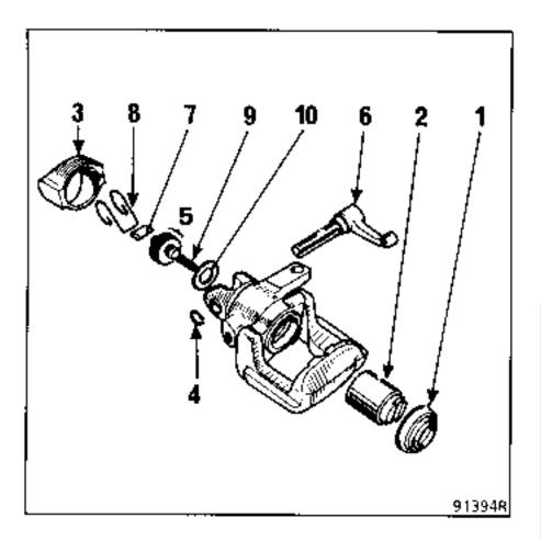
Compress flexible washers (5) using tool Fre. 514.
