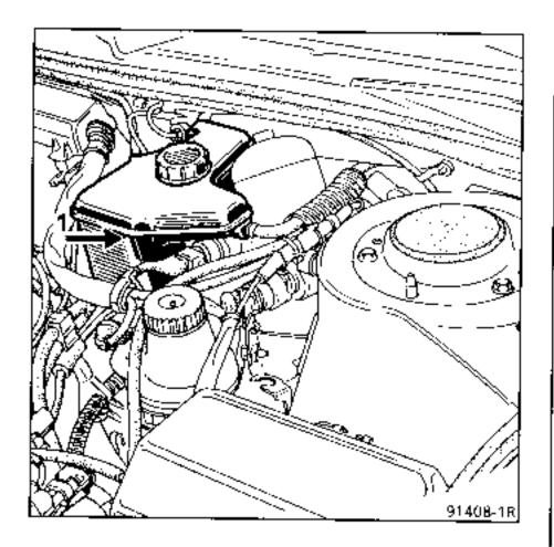
NOTE: The brake fluid reservoir capacity is designed to compensate the liquid from the accumulator when it has been emptied.
