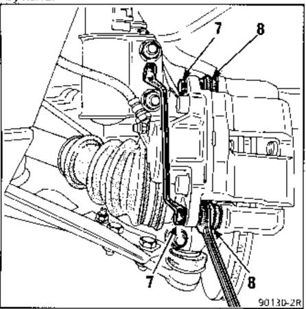
Remove the guide bolts (7) using two spanners.
