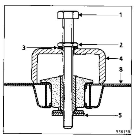
Fit threaded washer (5) between cradle (8) and chassis (9).
