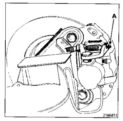
Gradually tension the cables at the central adjustment point so that end piece (A) comes into contact with the lever but does not move it.
