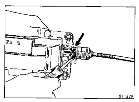
On reassembly, assemble the cable on the casing. (Place the key in the correct direction.)
