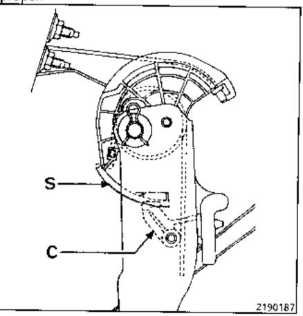
This device consists of a spring - activating capsule assembly located between the clutch pedal and the pedal assembly mounting.
