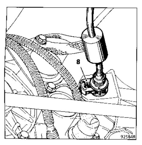
Under the floor engage the control unit equipped with its seal.
