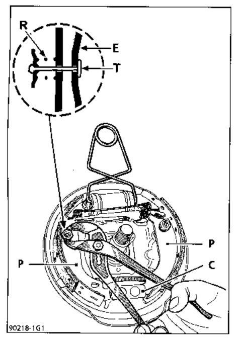
Pass each shoe base (P) above fixed point (C). alternately. Tighten the shoe bases with respect to one another to move the tips away at the wheel cylinder.
