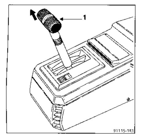
Remove the console embellisher pressing on the left-hand side and raise it to free the grips.
