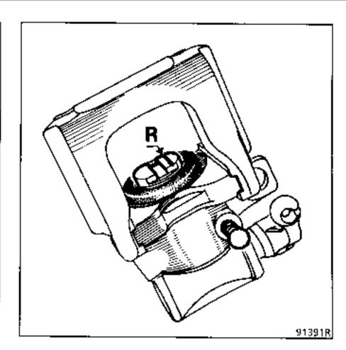
Coat the periphery of the piston with **SPAGRAPH** grease.
