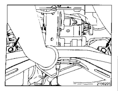
Remove the steering box from the lefthand side inner wing panel side.
