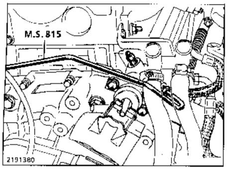
Check the travel of the slave cylinder. It should be:
