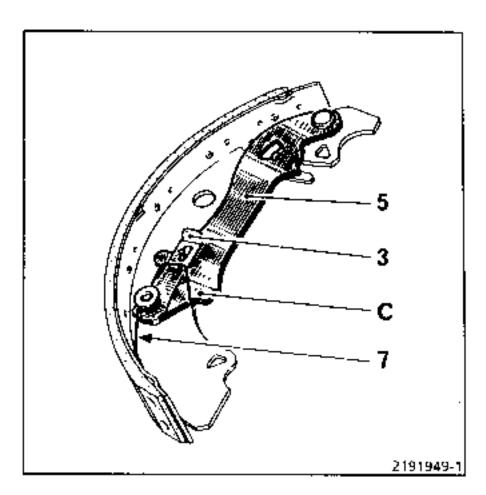
Check that the spring is correctly positioned (7).
