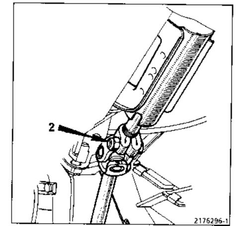
Disconnect the steering ball joints using tool T.Av. 476.
