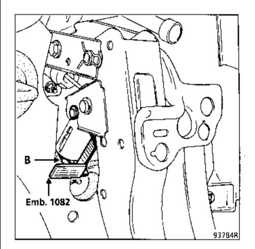
Remove the circlips and shaft (B).
