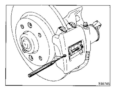
Refit rollpin (T) and the handbrake cable.
