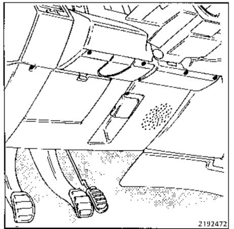
Fit tool Emb. 1082 in place of the spring activating capsule assembly.
