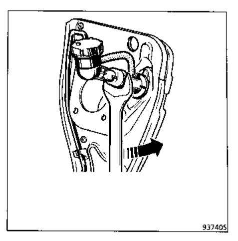
Check that the position of the markings of the master cylinder and plate are opposite one another.
