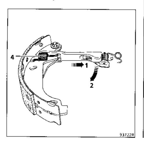
Marking and reassembly of the parts constituting the RAI system.
