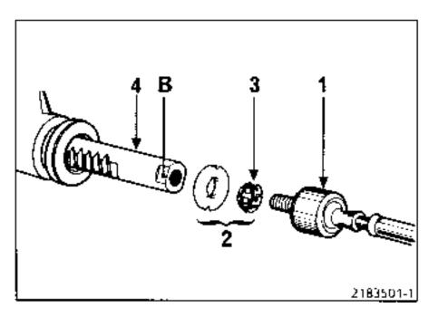
NOTE : Make sure that the two tabs on lock washer (2) are in line with flats (B) on the rack before tightening with wrench tool Dir. 812-01 or Dir. 832-01
