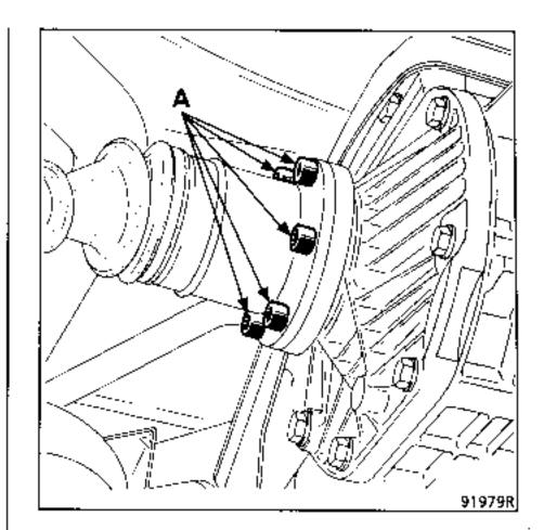
Disengage the drive shaft from the sun wheel and leave it suspended.
