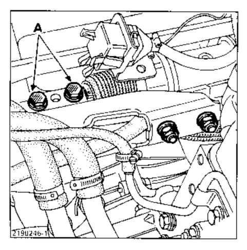
NOTE : As the steering rack nose has threaded bolt holes, the lock nuts must first be removed from bolts (A).
