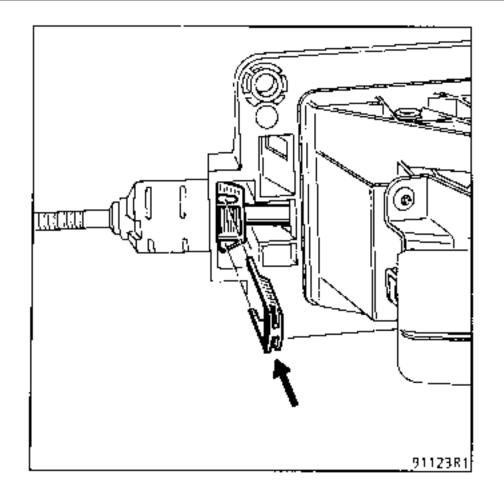
Clip the ball joint on to the base of the lever.
