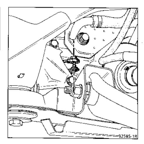
Align the cable ball joint with the ball joint on the gearbox lever, adjusting the position of the sheathing.
