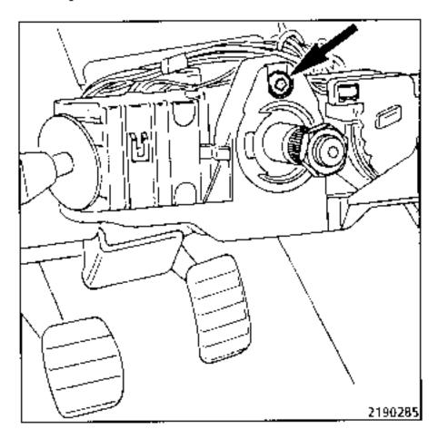
bolt (2) securing the intermediate shaft and the steering wheel shaft.
