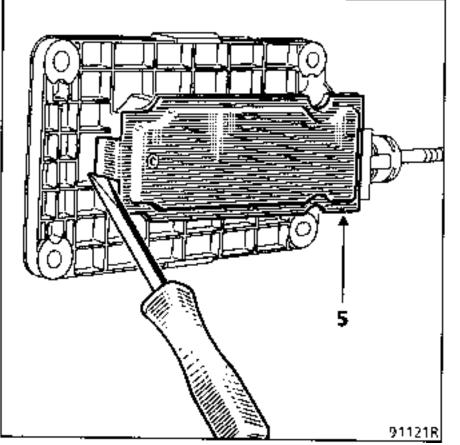
Unclip the ball joint from the base of the lever.
