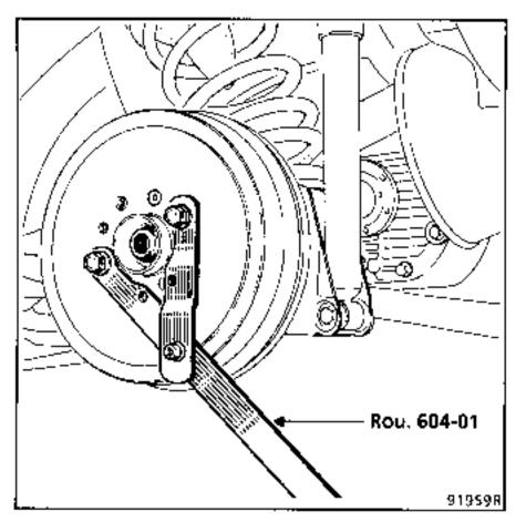
Remove the six bolts (A) securing the drive shaft on the sun wheel.
