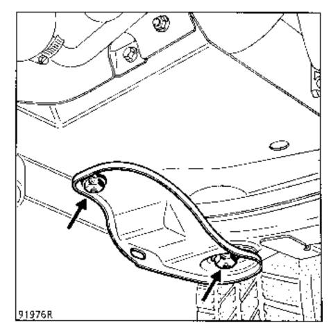
Lower the strut, disengaging the prop shaft from the cross member.
