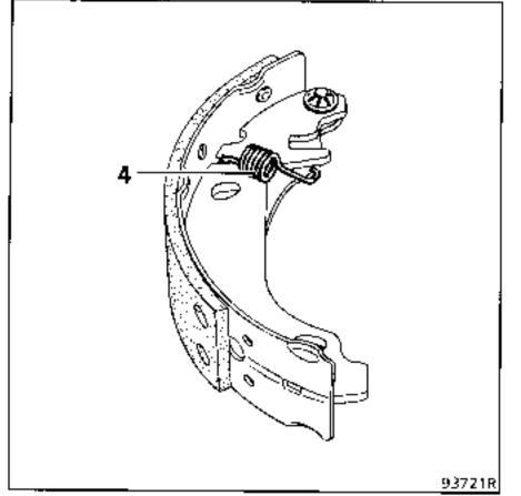
Attach the RAI assembly to spring (4) then pull in the direction shown by the arrows and the RAI moves automatically into its operating position.
