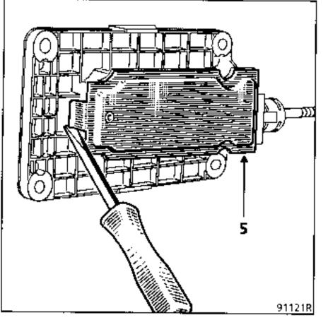
Unclip the ball joint from the base of the lever.
