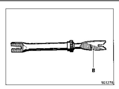
On the right-hand brake: the screw thread is lefthand.
