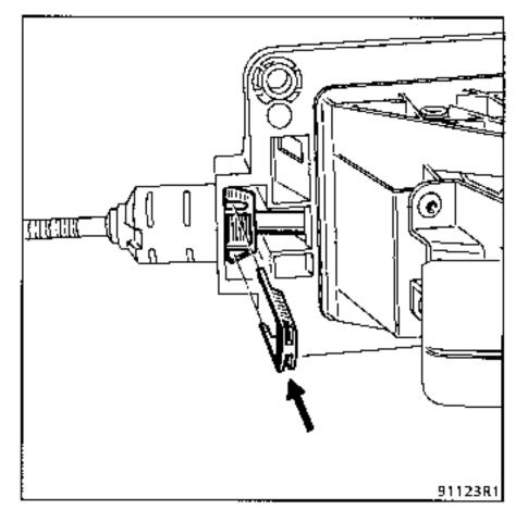
Clip the ball joint on the base of the lever.
