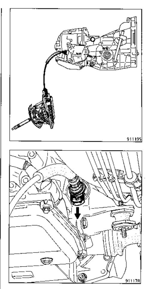
Under the floor panel, engage the control unit equipped with its seal.
