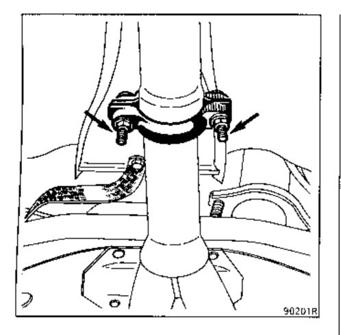
the gear selector control from under the lever, marking its position.
