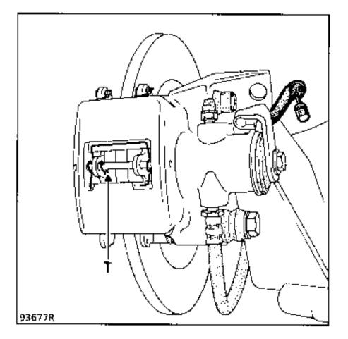
Press down on the brake pedal several times in order to bring the piston into contact with the pads.
