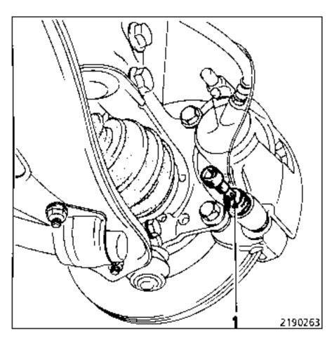
Unscrew guide bolt (1) and separate it from the calliper bracket.
