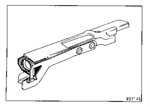
Then assemble the link arms with their respective bolts and nuts, with the right-hand bolt, clip and nut in the right-hand link arm, passing through the hole in the bracket and likewise for the lefthand RAI.
