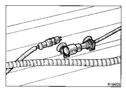
If the ABS warning light illuminates intermittently, check first of all the wheel sensor connectors and clean them with **NETELEC**, **Part No. 77 01 408 464**.
