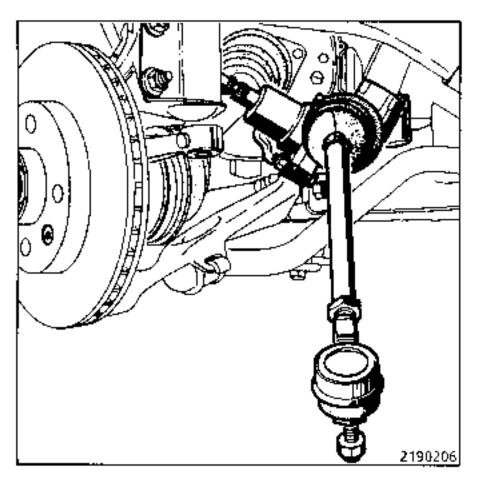
The axial ball joints must only be unscrewed from the rack if they are going to be changed.
