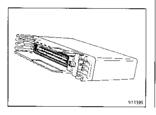
It analyses the data from the wheel sensors and controls the inlet and outlet solenoid valves according to this data.
