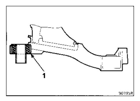
Fit in place the bearing on the bush ensuring dimension  $X = 24 \pm 1 \text{ mm}$  between the bearing face and stub axle shaft.
