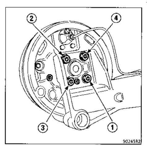
NOTE: If the stub axle mounting bolts are re-used, they must be smeared first with LOCTITE FRENBLOC or a new spring lock (grower) washer must be fitted.
