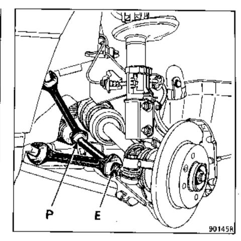
Disconnect the steering arm ball joint using tool T.Av. 476.
