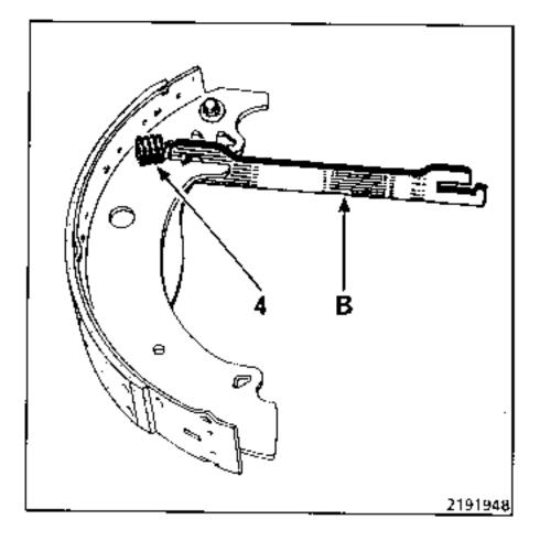
Remove the wear compensation lever (5) from the leading shoe.
