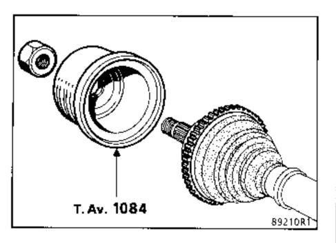
NOTE: In future, the Parts Department will only supply in service exchange machined drive shaft not equipped with the anti-lock braking sensor targets. The sensor targets must therefore be retained in order to be realigned on the drive shafts. The sensor targets alone, however, are available from the Parts Department.
