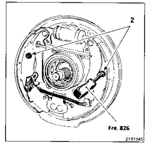
Fit a grip on the wheel cylinder pistons.
