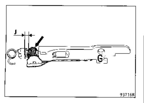
Note the **G** (left-hand) stamped on the part and the position of the bracket.
