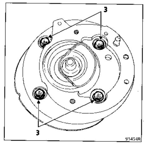
DISMANTLING THE SPRING AND SHOCK ABSORBER
