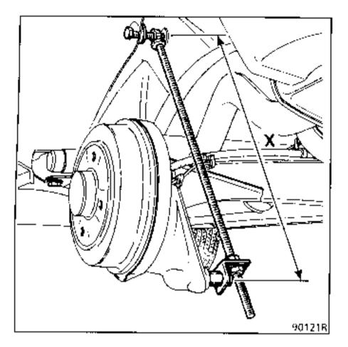
The bearings have a mark (1) enabling the suspension bars to be initially positioned, but mark (2) must be made on the external anchorages of the anti-roll bars.
