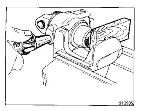
Take the seal out of its groove using a steel blade with rounded edges.
