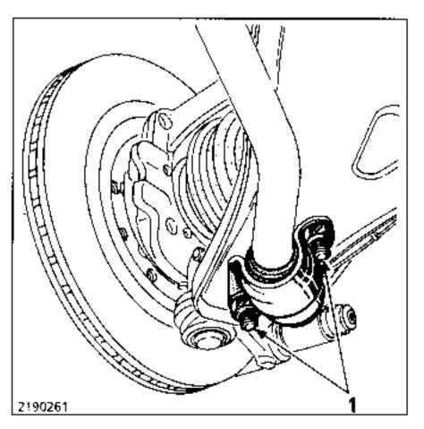
NOTE : The bolts securing the bearing (1) also hold the lower ball joint, so place a nut on one of the bolts to prevent the lower ball joint slipping.
