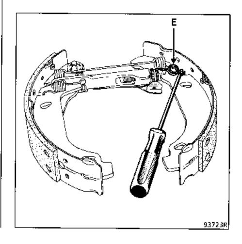
Pivot leading shoe (A), as shown by the arrow so as to release the head of the RAI screws. This will enable upper spring (1) to be removed easily.
