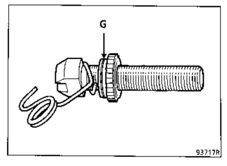
The bolt has a left hand thread, the notched nut has a groove (G) and the clip is not painted.
