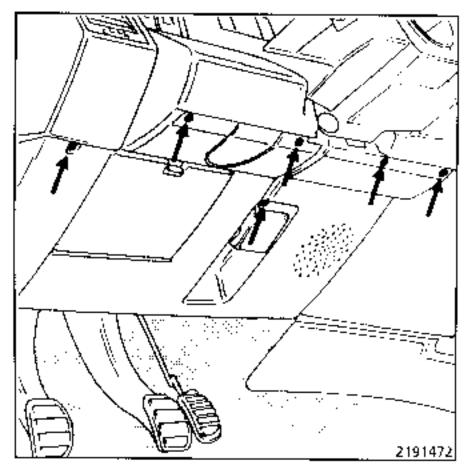
NOTE: To remove the cover under the steering wheel on vehicles of the first type, the glovebox must be opened.
