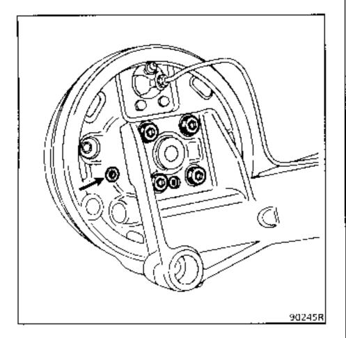
Insert a screwdriver and push against the handbrake lever to release stud (E) from the brake shoe.
