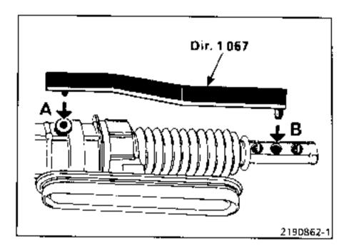
In this position, fit the measuring equipment and check the parallelism.
