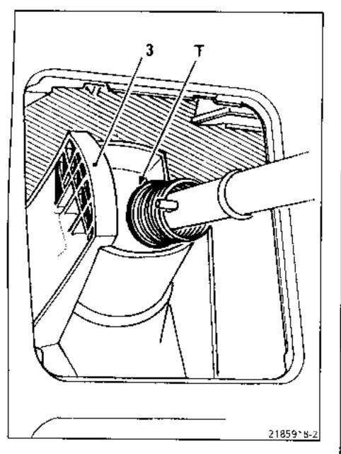
Note: In order to prevent the parts returning automatically to the earlier setting, it is sometimes necessary to turn the lever clevis in the connection rod. Leave a space of 5 mm between the connecting rod and the clevis.
