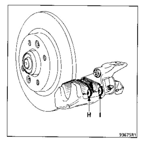
**NOTE :** On some vehicles the bolt mounting the main carrier (E) must be slackened in order to remove inner pad (I).
