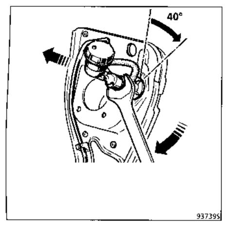
Free the hose line from its mounting on the plate and remove it together with the master cylinder.
