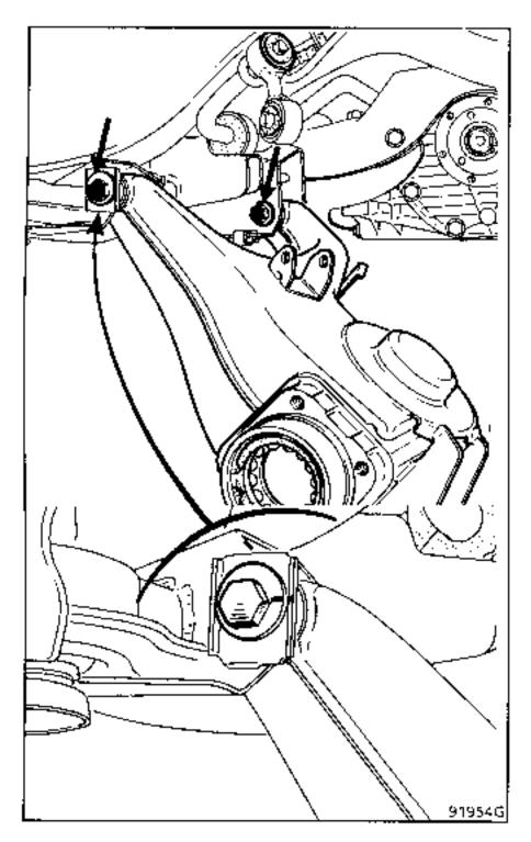
Fit a jack under the arm and fit the spring (see the instructions in the relevant paragraph).
