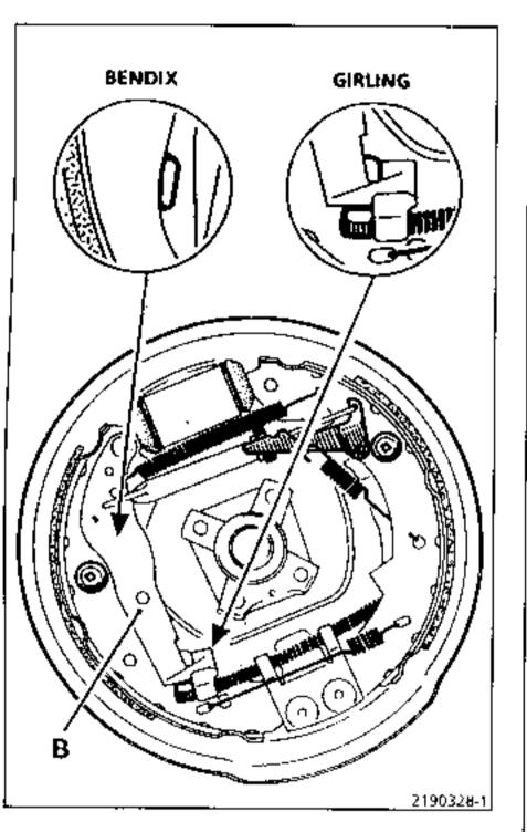
Gradually tension the cables at the central adjustment point so that levers (B) lift off between the 1st and 2nd notches of the control lever travel and stay lifted off at the 2nd notch.
