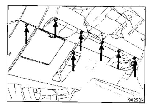
NOTE: On vehicles of the 1st type, the glovebox must be opened in order to remove the cover under the steering wheel.
