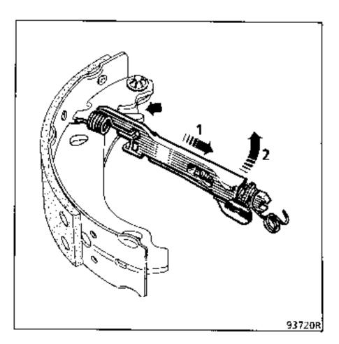
Position the upper spring (1) in the notches in the two shoes, then pull in the direction shown by the arrows and the recess on the bolt should locate in that of the leading shoe (A).
