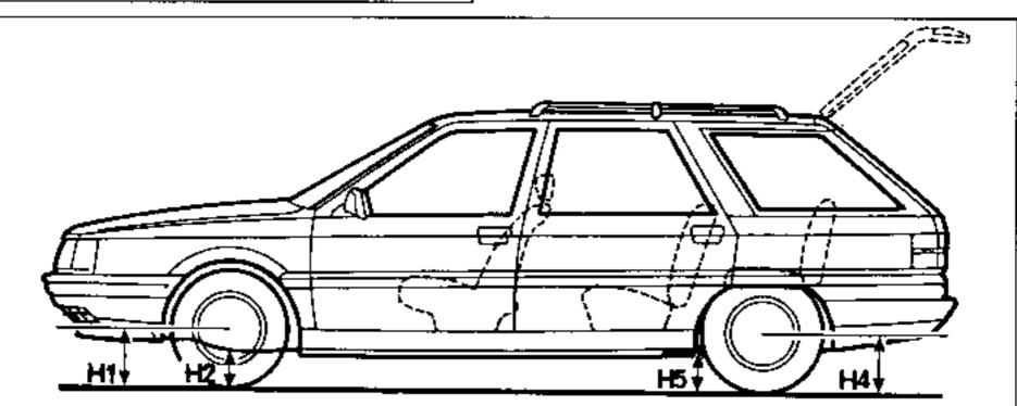
The underbody height is measured with the vehicle unladen (preferably on a lift) :
