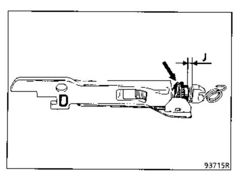
Note the D (right-hand) stamped on the part and the position of the bracket.
