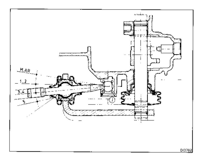
Under the vehicle: disconnect spring (2) then slacken bolt (V) securing the clip to connecting rod (1).
