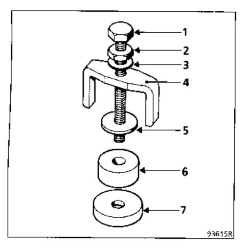
The extraction operation is performed using parts (1), (2), (3), (4), (5).
