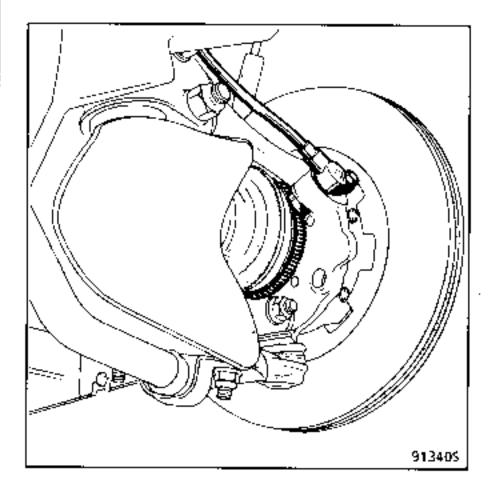
For the rear wheels, the targets are press-fitted on the hubs (cannot be dismantled).
