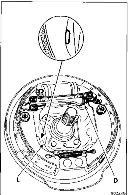
Gradually tension the cables at the central adjusting point so that levers (L) lift off between the first and second notches of the control lever travel and remain lifted off at the second notch.
