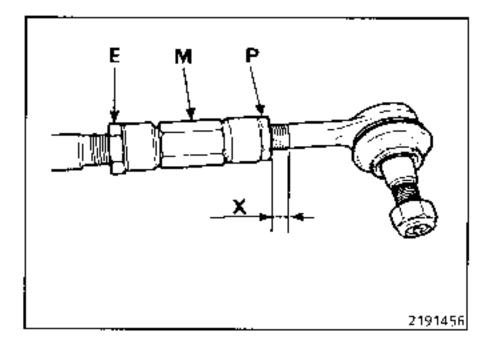
Reconnect the ball joint in the stem of the shock absorber.
