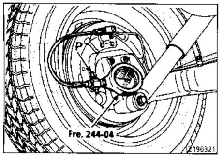
Operate the brake pedal progressively until the correct pressure setting is obtained on the front wheels (see table).
