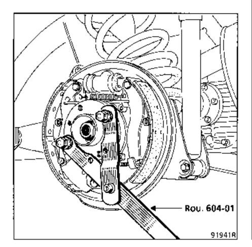
the six mounting boits (A) on the sun wheel, with the hub locked in place, using tool Rou. 604-01.
