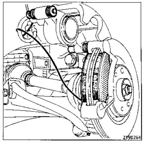
fit the calliper on its upper guide and tilt it downwards.
