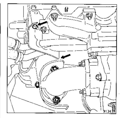
Disconnect the feed hose from the slave cylinder.
