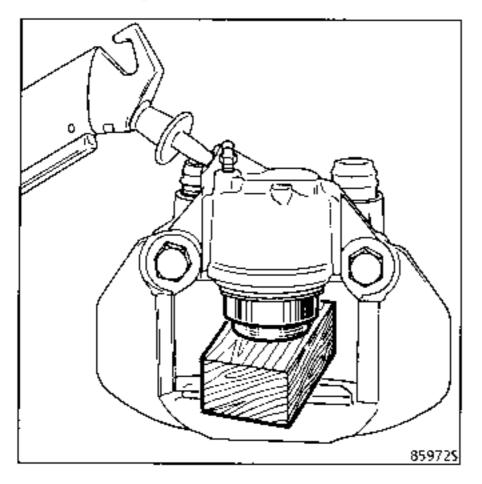
Take out the rectangular section seal from the calliper groove using a round-ended flexible blade (eg, a feeler gauge).
