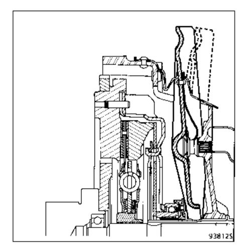
It is **not permissible** to top up the fluid. The unit is supplied as two units (master cylinder and slave cylinder) and is already filled with fluid.
