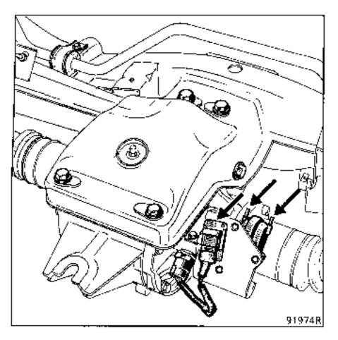
the rear mounting for the final drive on the body,
