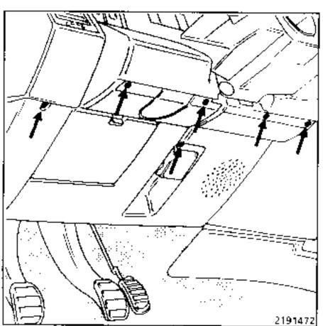
NOTE: On the 1st type, the glove compartment must be opened to remove the cover under the steering wheel.
