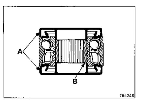
On the press, fit the bearing with its plastic ring (B) in the stub axle carrier using a piece of tubing with an outer diameter of 71 mm and a bore of 66 mm, resting on the outer track bearing.
