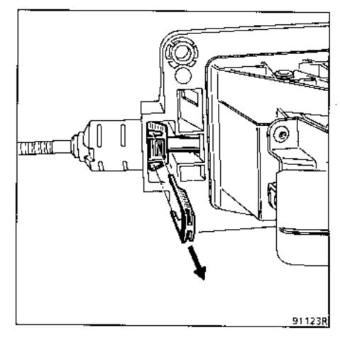
Free the cable by pressing on the two locking catches in the casing.
