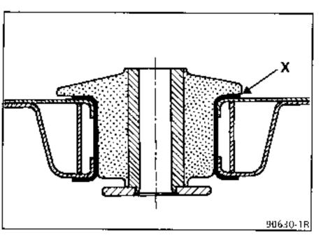
X = 0.3 mm : maximum clearance after fitting between studs and cradle.
