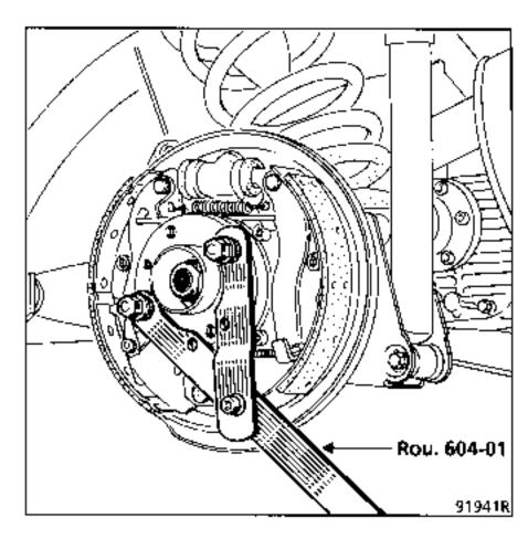
Push back the drive shaft to release tools T.Av. 1050-02 + Rou. 604-01.
