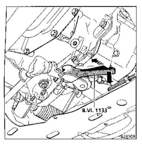
At the same time, pull the end of the tool downwards and pivot it through approximately **45°** until it is up against the spur on the casing. Fit connecting rod (1) on lever clevis (5), leaving a space of approximately 5 mm between the connecting rod and clevis.
