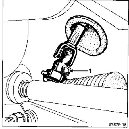
the collapsible steering wheel shaft.
