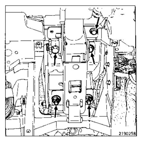
Disconnect the steering lock switch and remove the steering column.
