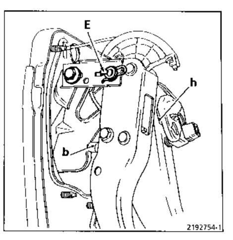
**NOTE :** From now onwards the stiffener has a locking spur (E) preventing all risk of the shaft moving.
