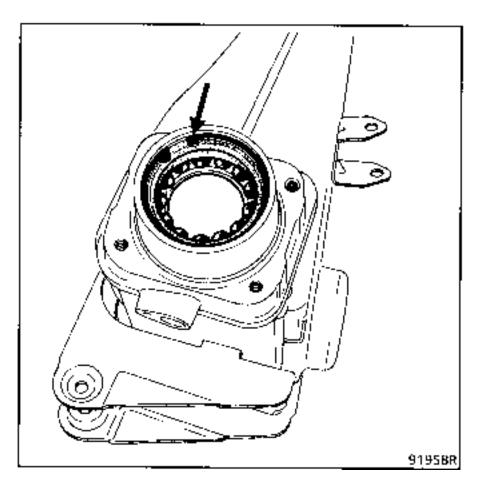
On the press, extract the outer track ring using one of the two inner track rings, leaving the ball races and seals in position.
