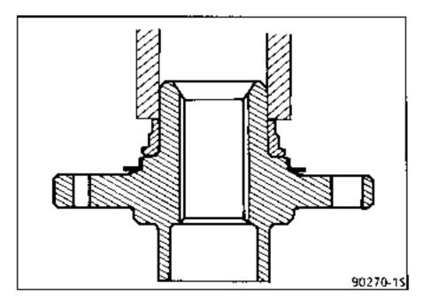
Coat the ball bearings, the bearing tracks and sealing lips with grease.
