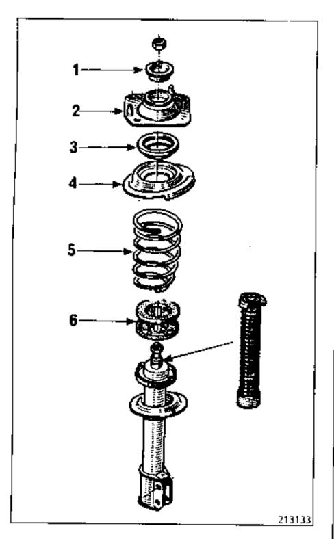
Parts 3 and 4 form the stub axle carrier pivot assembly.
