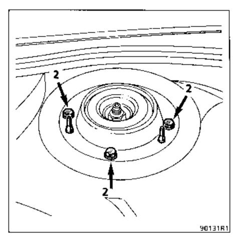
the shock absorber, pressing down on the bottom arm to prevent the shock absorber coming into contact with the driveshaft gaiter.
