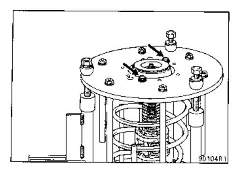
the three compression bolts, putting plenty of oil in the oil grooves.
