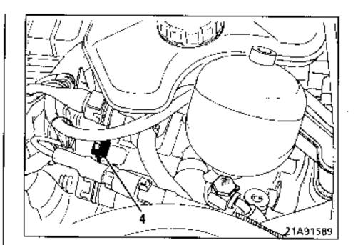
the power assisted steering fluid chamber.
