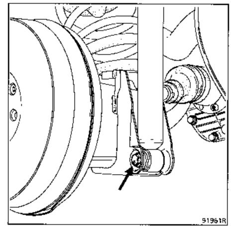
the mounting from the anti-roll bar link arm.
