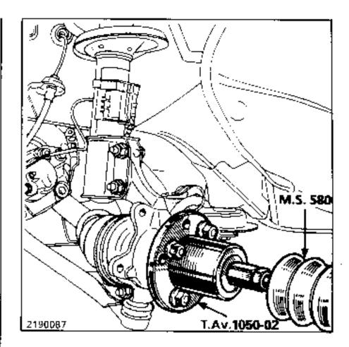
Remove the interior bearing ring using the hub bearing extractor kit, see Tooling Catalogue, tool reference 914 0951.
