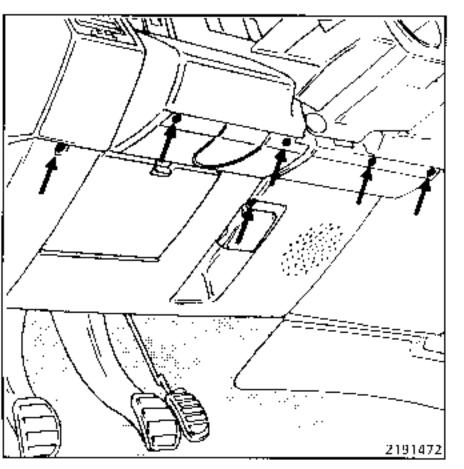
NOTE : To remove the cover under the steering wheel on type 1 vehicles, the glove compartment has to be opened.
