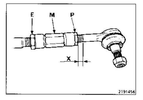
When adjusting the parallelism, ensure that the lengths X of the ball joint housings on the steering arms are symmetrical.
