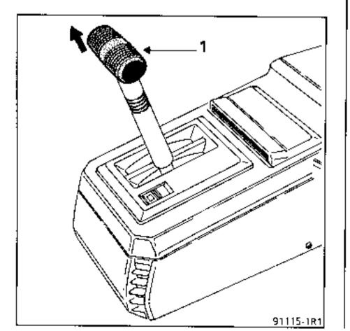
Remove the console embellisher pressing on the left-hand side and raise it to free the grips.
