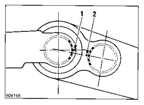
To do this: place a ruler on the centreline of the two anchorages and make a mark (2) (at the bottom of a tooth).
