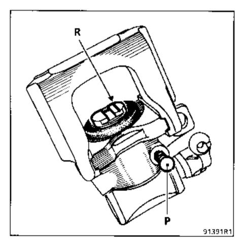
Direct the piston so that line (R) on its bearing face is at bleed screw (P) end.
