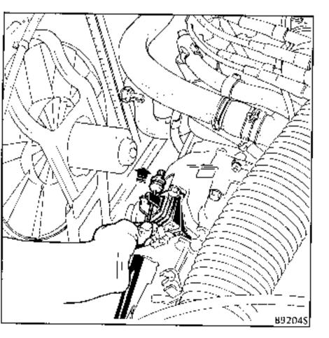
These checks enable you to check that notched cam (C) and toothed sector (S) are free in the "clutch engaged" position.
