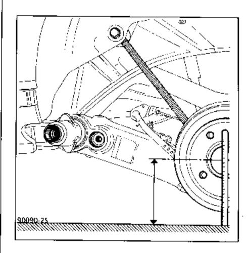
Then, by moving both tools, decrease or increase the distance between the centre line and the ground at the same time on both sides by the difference in height measured when the vehicle was checked.
