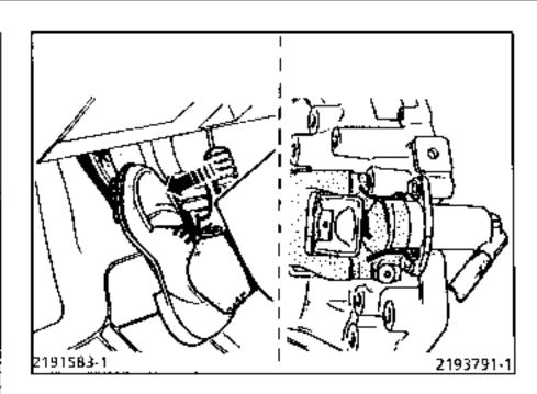
Press down fully on the clutch pedal and allow it to return gently to its top stop (2 or 3 times).
