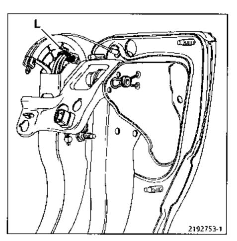
Fit the cable in place at the fork end.
