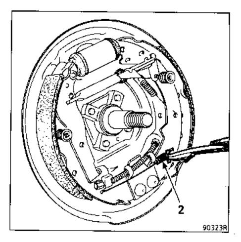
Fit clamp to the wheel cylinder piston.
