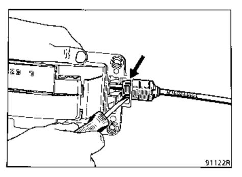
On reassembly, assemble the cable on the casing. (Ensure the key is placed in the correct direction.).
