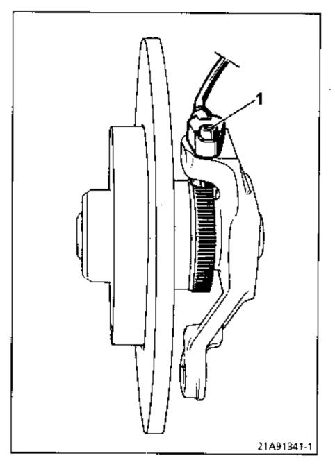
Unclip the lead from its mounting.
