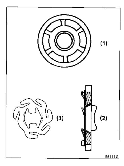
**REMOVING THE BALL JOINT :** Assembly (2) must be changed systematically at each dismantling. The ball joint itself may be used again if the notches are undamaged.
