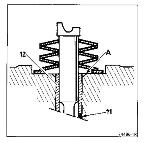
Check the position of the flexible washers: they must be fitted as shown in the diagram to allow the handbrake lever to be in the "rest" position.
