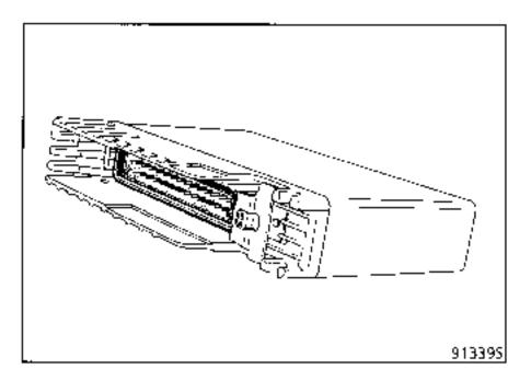
It continuously tests all its peripheral units; if it detects a problem, it instructs warning light to illuminate.
