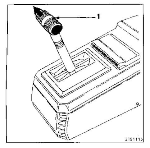
Remove the console embellisher by pressing on the left-hand side and raise it to free the grips.
