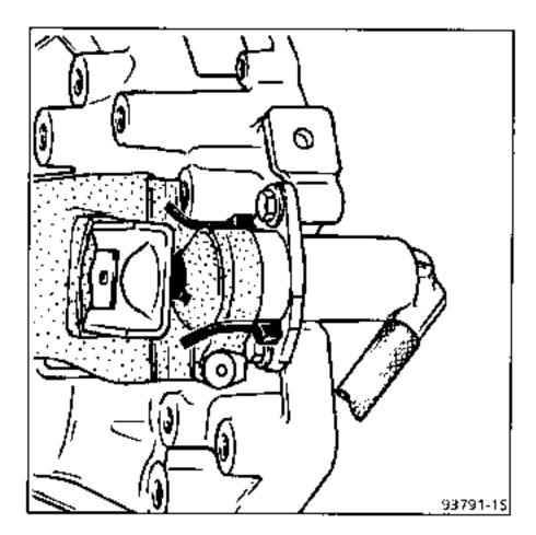
Move the hoses away and remove the slave cylinder.
