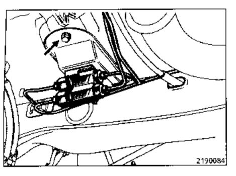
Tilt the support - compensator assembly then remove it.
