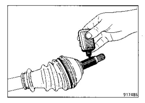
Engage the hub on the driveshaft stub axle (using a mallet if necessary) until the nut can be screwed up by a few threads.
