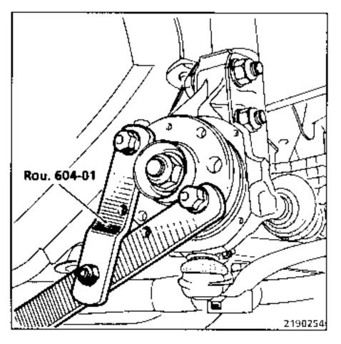
Through holes (B) in the hub, remove the bearing securing bolts.
