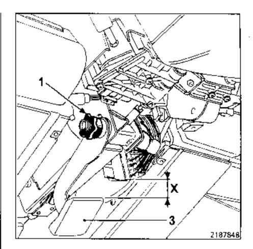
Lock the steering column by tightening nut (2) using locking lever (3).
