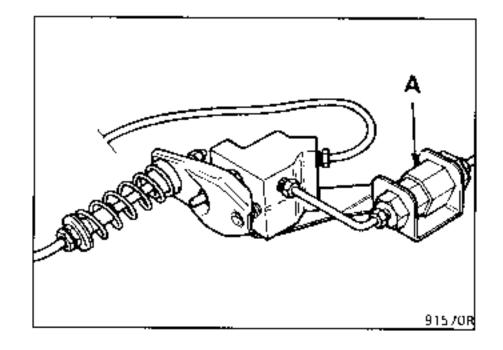
This valve enables the increase in pressure on the rear axle to be slightly offset.
