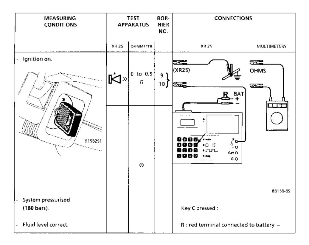
© If incorrect: check continuity between terminal (9) of computer, terminal (1) of connector A, terminal (2) of connector A, terminal (3) of connector D (105 bar switch pressostat), terminal (5) of connector D and terminal (10) of computer.
