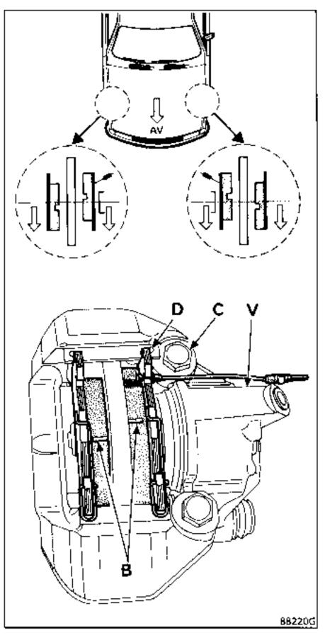
Position the pads in the calliper and insert wedge (2).
