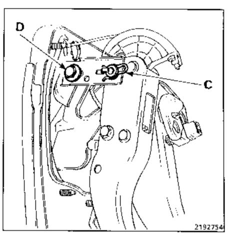
Slacken bolt (D) and release the stiffener.
