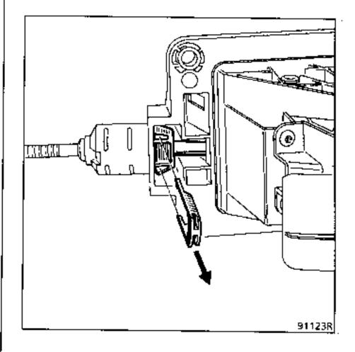
Release the cable by pressing on the two locking catches in the casing.
