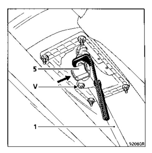
In this position, tighten bolt (V).
