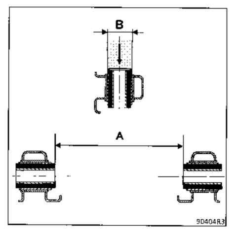
$B = \emptyset$  **30** transverse engine  $B \simeq \emptyset$  **34** in-line engine
