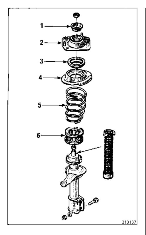
Parts 3 and 4 form the stub axle carrier pivot assembly.
