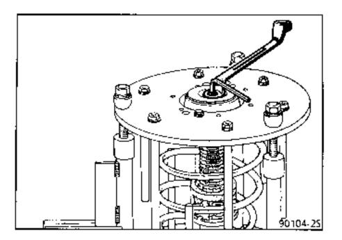
Torque tighten the nut.
