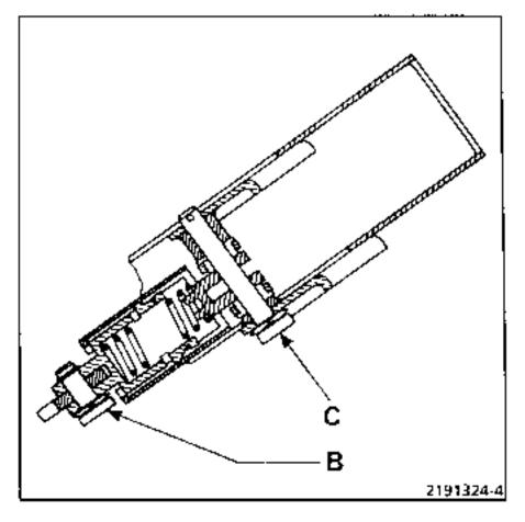
Fit the pushrod calliper (equipped with its plastic bearings) between the spring - activating capsule assembly and the pedal.
