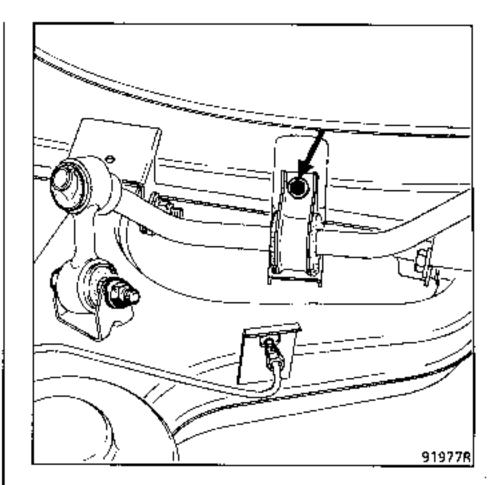
Take out the bar on the left-hand side, directing it as shown in the drawing.
