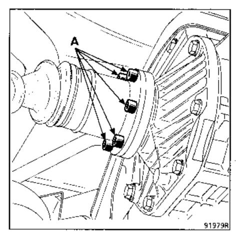
Push back the drive shaft and recover it using tools T.Av. 1050-02 + Rou. 604-01.
