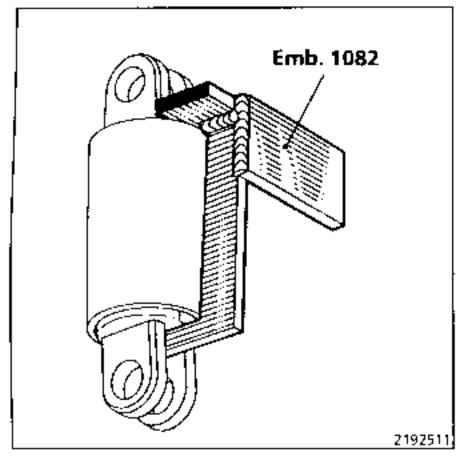
Fit the parts the correct way round: the section of the capsule with the larger diameter must be at the pushrod end).
