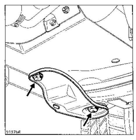
**NOTE:** If the final drive mounting cross member is being replaced, remove the anti-roll bearings.
