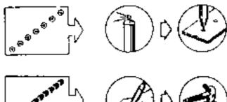
1 M.A.G. welding fillet 90 mm long 2 M.A.G. welding fillets 15 mm long
