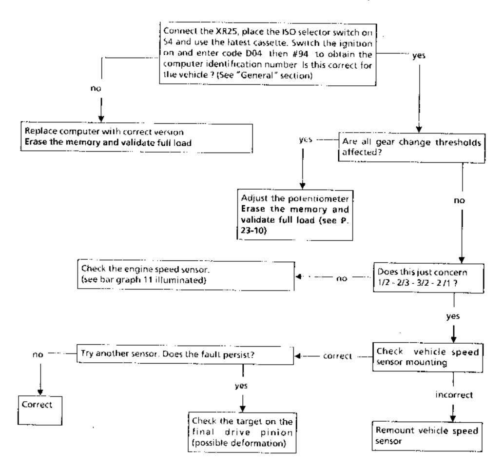
IMPORTANT : DO NOT FORGET TO ERASE THE MEMORY AND VALIDATE THE FULL LOAD POSITION (see P. 23-10)
