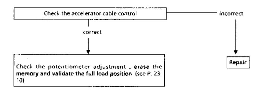
IMPORTANT : DO NOT FORGET TO ERASE THE MEMORY AND VALIDATE THE FULL LOAD POSITION (see P. 23-10)
