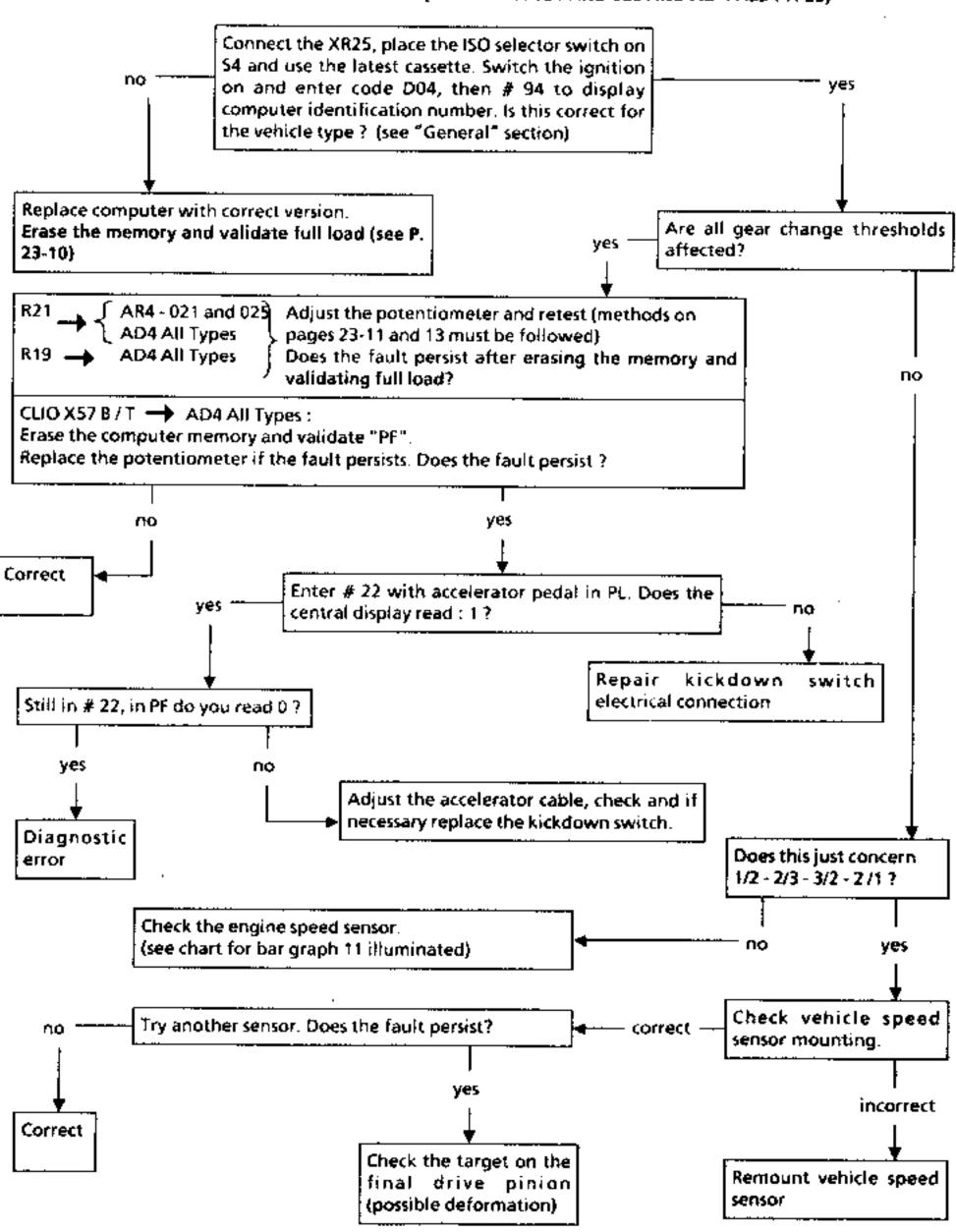
FAULT: GEARS DO NOT CHANGE, "AT" LOCKED IN ONE GEAR, WARNING LIGHT ILLUMINATED
