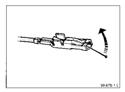
If the tool falls out, the connection is faulty. Carefully retighten the connector using a needle or paper clip.
