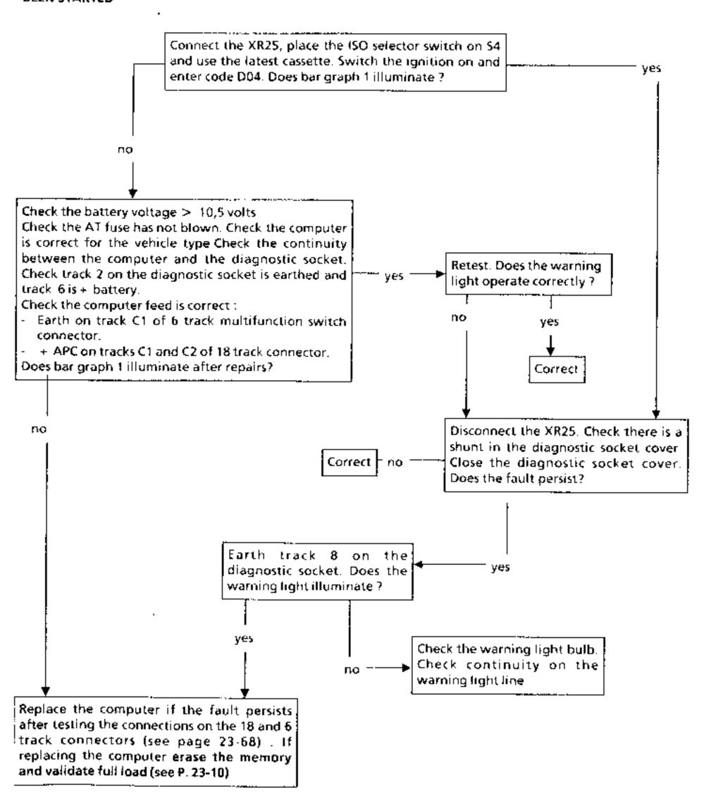
FAULT: FAULT WARNING LIGHT PERMANENTLY ILLUMINATED WHILE DRIVING, PERSISTS AFTER ENGINE STARTED AGAIN, WITHOUT AT FAULT.
