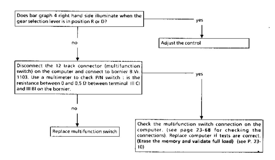
IMPORTANT : DO NOT FORGET TO ERASE THE MEMORY AND VALIDATE THE FULL LOAD POSITION (see P. 23-10)
