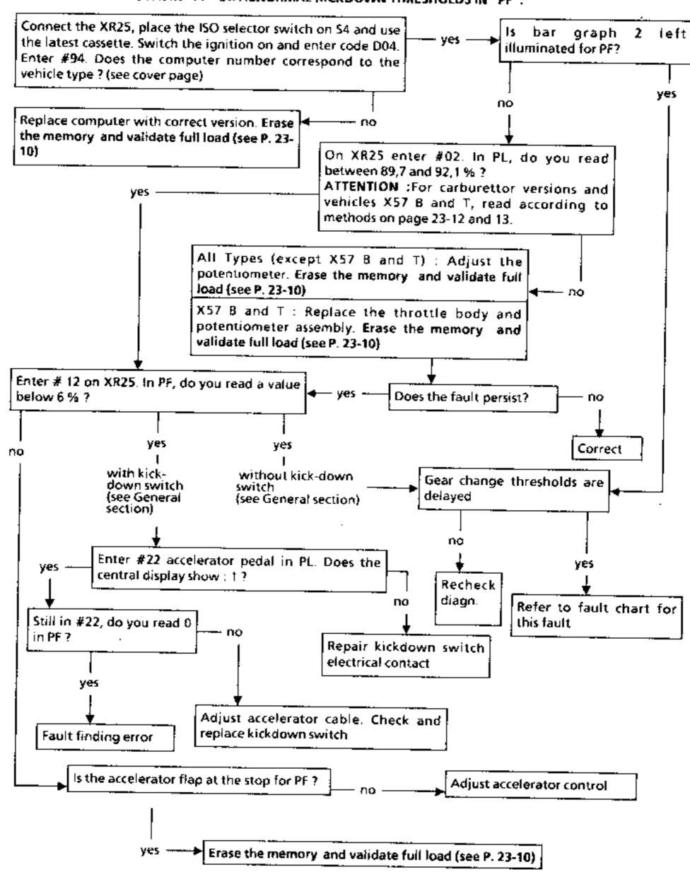
FAULT: GEAR CHANGE THRESHOLDS DELAYED WHEN ENGINE HOT ONLY OR WHEN ENGINE COLD ONLY, WARNING LIGHT EXTINGUISHED.
