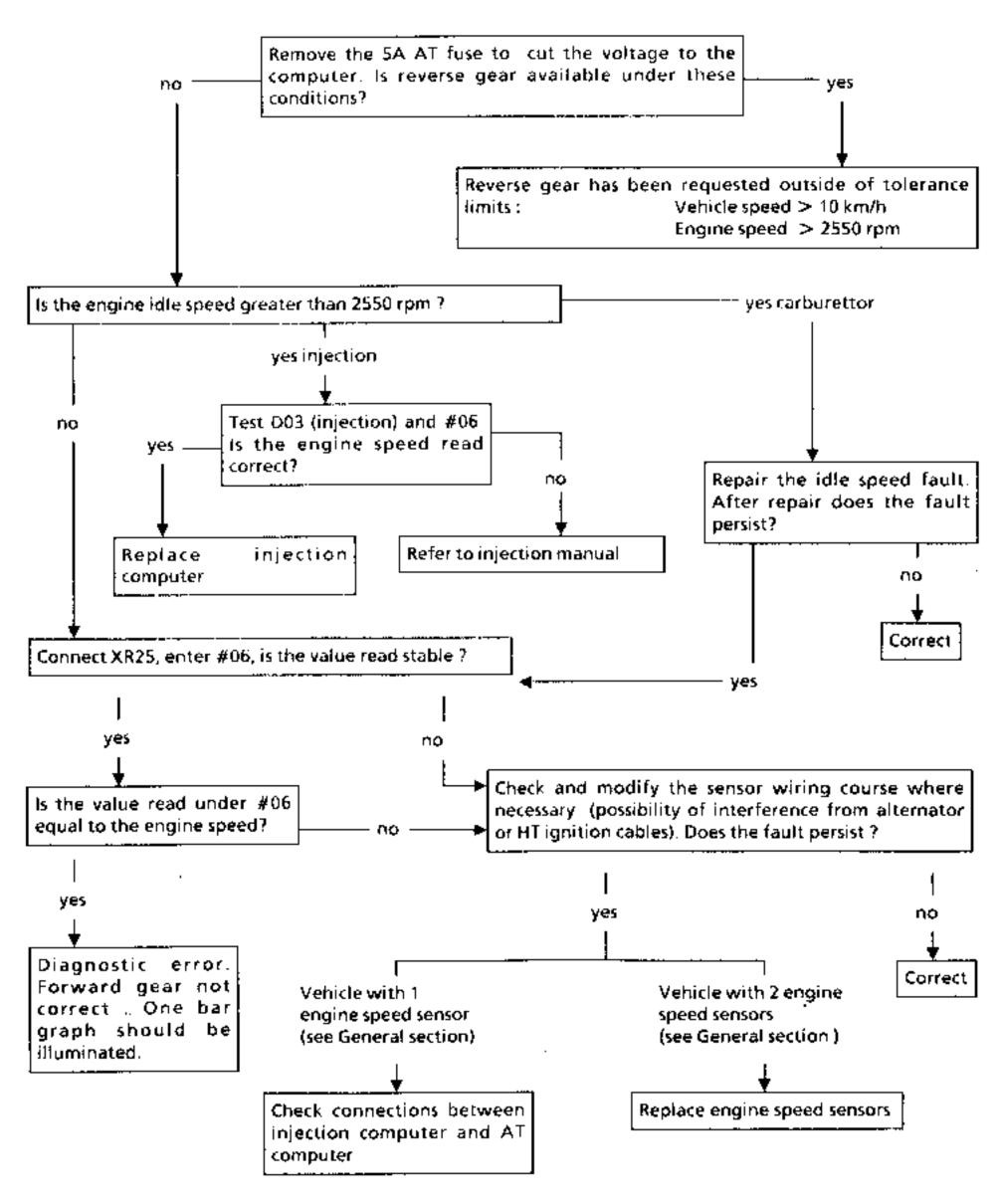
FAULT: PRESENCE OF CHANGING UP OF GEARS WHICH ARE NOT AUTHORISED BY THE GEAR LEVER POSITION, WARNING LIGHT EXTINGUISHED.
