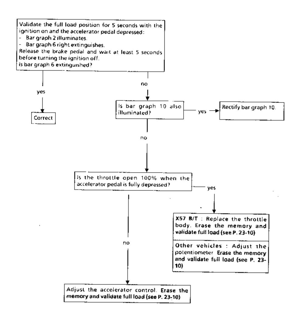
FAULT: BAR GRAPH 7 ILLUMINATED. (Fault on multifunction switch)
