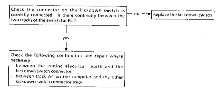
Bar graph 2 right extinguished for PF Earth on track A4 of computer .
