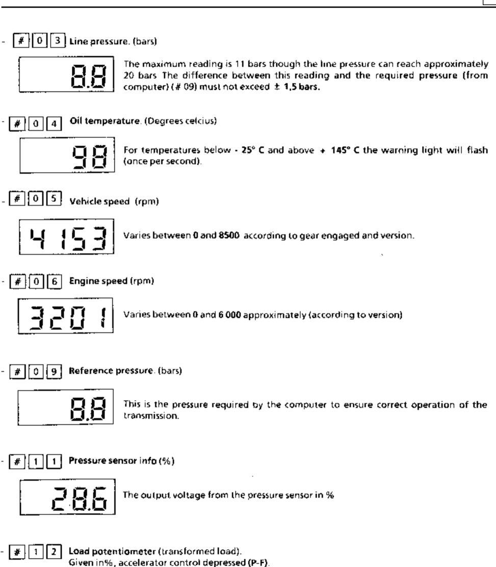
Value less than 6%, accelerator pedal depressed completely (for kickdown).
