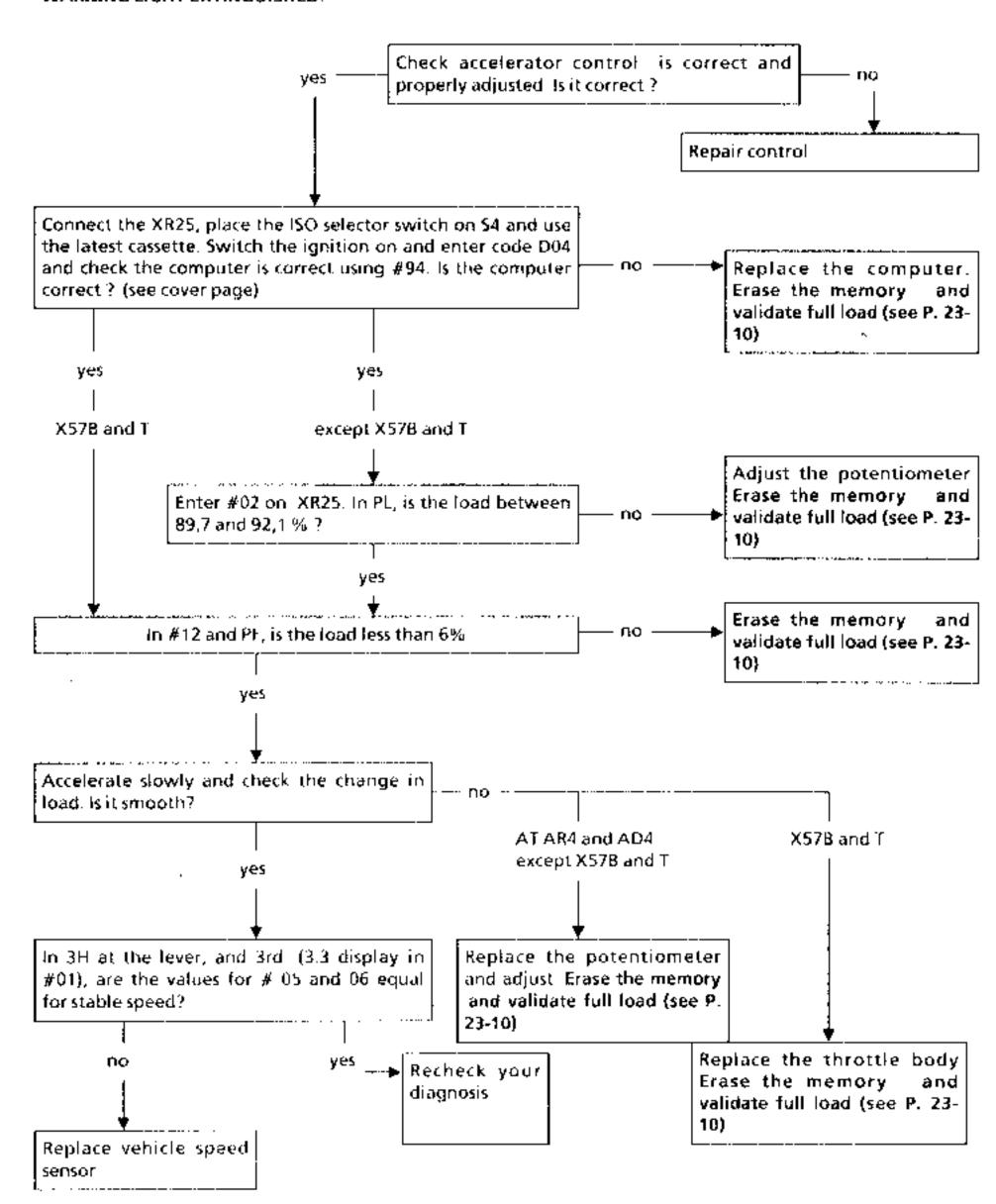
FAULT : JERKY OPERATION, SLIPPING OR ENGINE RACING DURING GEAR CHANGE, WARNING LIGHT
