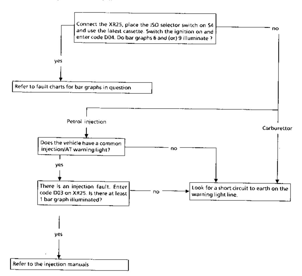
FAULT: FAULT WARNING LIGHT PERMANENTLY ILLUMINATED WHILE DRIVING, PERSISTS AFTER ENGINE STARTED AGAIN, WITH AT FAULT.
