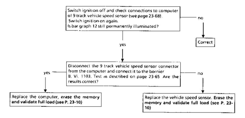
IMPORTANT : DO NOT FORGET TO ERASE THE MEMORY AND VALIDATE THE FUEL LOAD POSITION (see P. 23-10)
