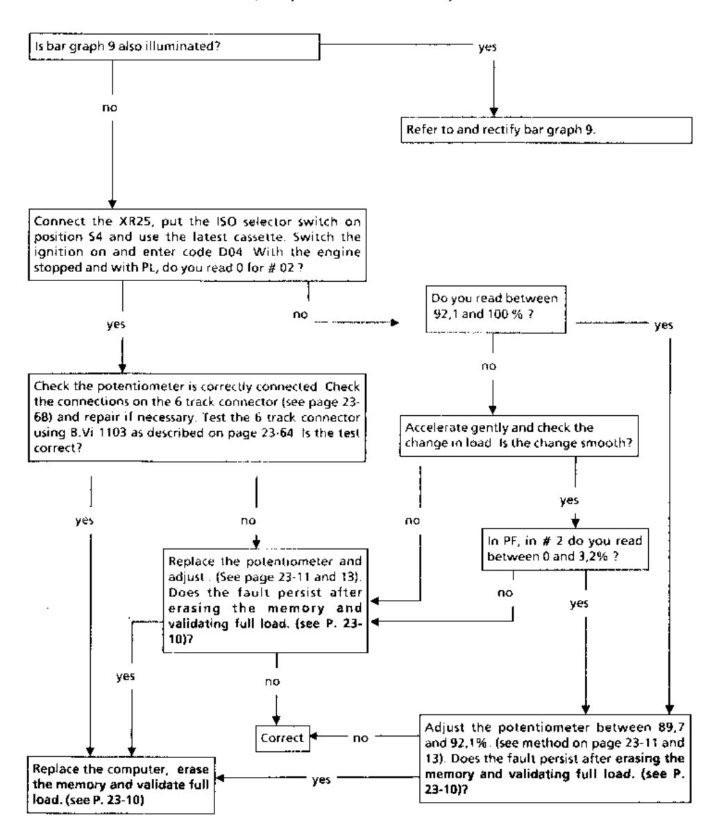
FAULT : BAR GRAPH 10 RIGHT ILLUMINATED (Load potentiometer circuit fault)
