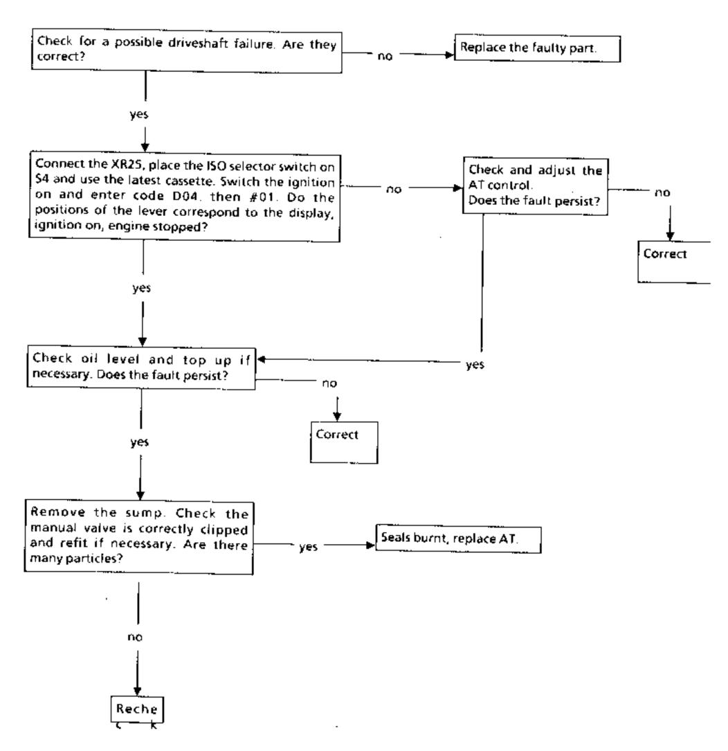
FAULT : NO DRIVE, WARNING LIGHT DOES NOT ILLUMINATE, ENGINE SPEED LIMITED TO STALLING POINT (APPROX. 2200 rpm)
