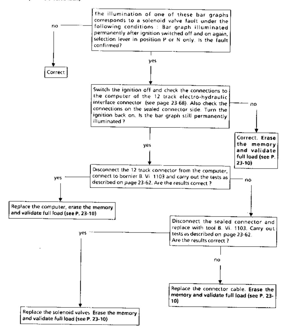
FAULT: THE WARNING LIGHT DOES NOT REMAIN ILLUMINATED FOR 3 SECONDS AFTER THE ENGINE HAS BEEN STARTED
