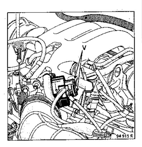
With the accelerator control in the rest position, turn the potentiometer body until the value on the display is between 89,7 and 92,1%
